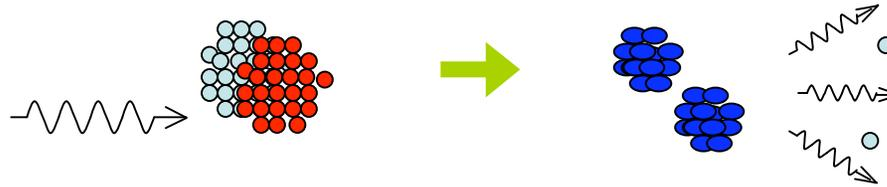
Nuclei are excited by gamma rays (Giant Dipole Resonance). If the nuclei are *fissionable*, one of the de-excitation channels is fission and fission fragments will decay emitting secondary gammas and neutrons. Because these secondary particles are from fission fragments, they come in a later time up to fractions of a minute. Detection of these *delayed* particles is a good signature of fission, or fissile material.
