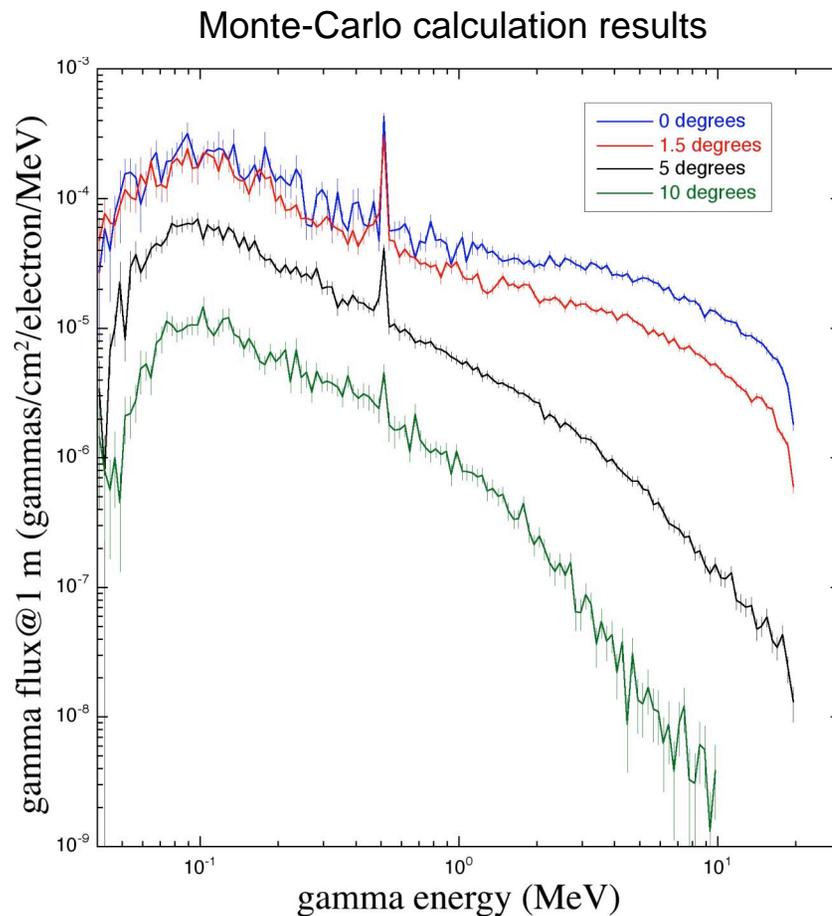
Bremsstrahlung with 0.1-mm tungsten target passed through a 30-cm Aluminum filter
