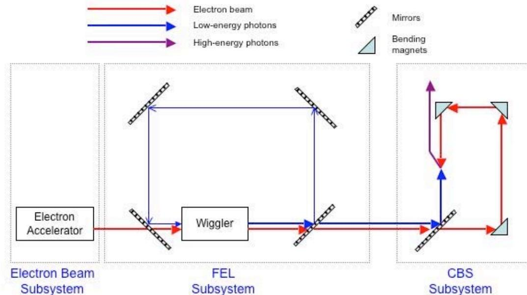
In a Compton source, low-energy photons collide with high-energy and upshift to high-energy gammas. Gamma energy is correlated with scattered angle.
