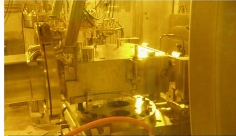
Target Change-out Test performed after mercury testing
