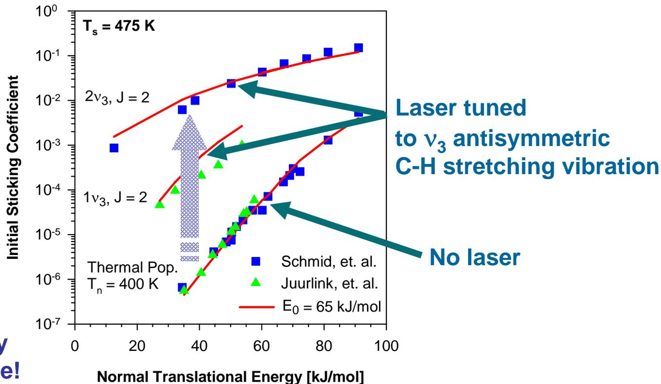
Dissociative chemisorption of a  $\text{CH}_4$  molecular beam incident on a Ni(100) surface with and without laser excitation.
