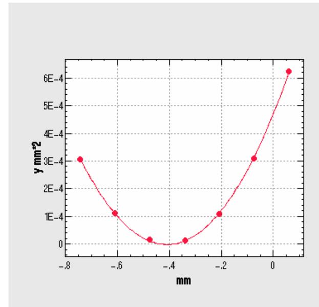
Beam Based alignment to determine all the BPM- to-quadrupole offsets
