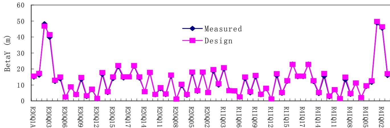
When the fudge factors were applied to the storage rings, it led to good agreement between theoretical and measured beam optics functions with  $\Delta\beta/\beta < \pm 10\%$ , at most quadrupoles, for tune:  $\Delta\nu < 0.002$ .
