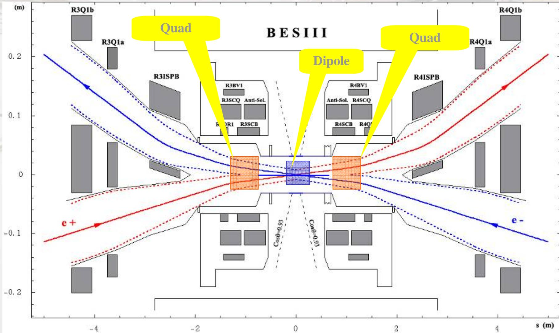
**Beam orbit in IR for the backup scheme**
