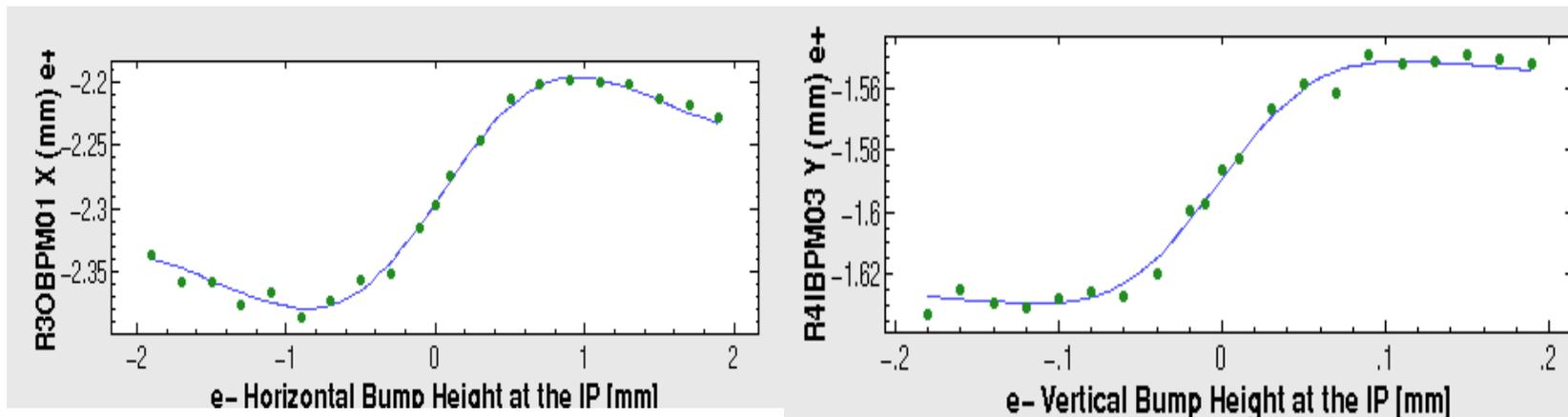
The beam size and IP position can be obtained by fitting the BBS data.
