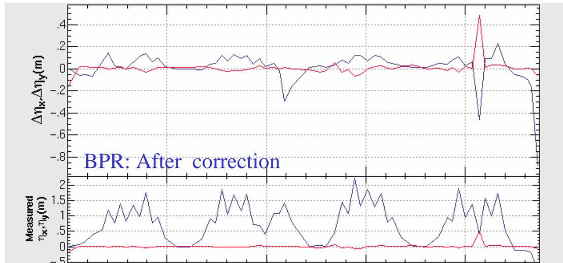
The deviation of measured dispersion function from the design is also small.
