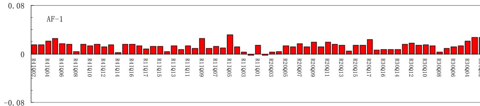
The fudge factors of quadrupole are mostly within 1.01~1.02, One possible cause of this systemic component may come from the short distance between the quadrupole and its adjacent sextupole. Other origin of these errors will be also pursued.
