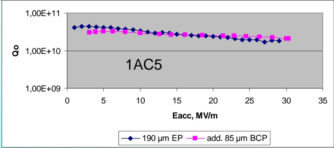
**Q(Eacc) curve of the single cell cavities 1AC3 -1AC5 after EP and BCP treatment**
