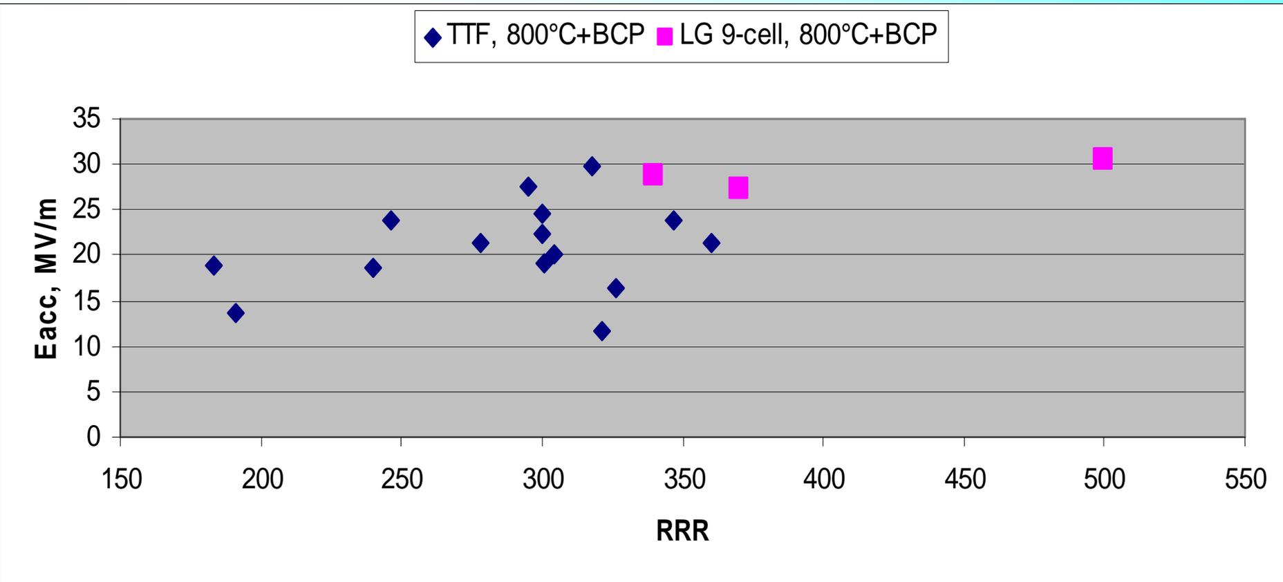
Comparison of the Eacc performance of large grain (LG) 9-cell cavities with similarly treated fine grain TTF cavities
