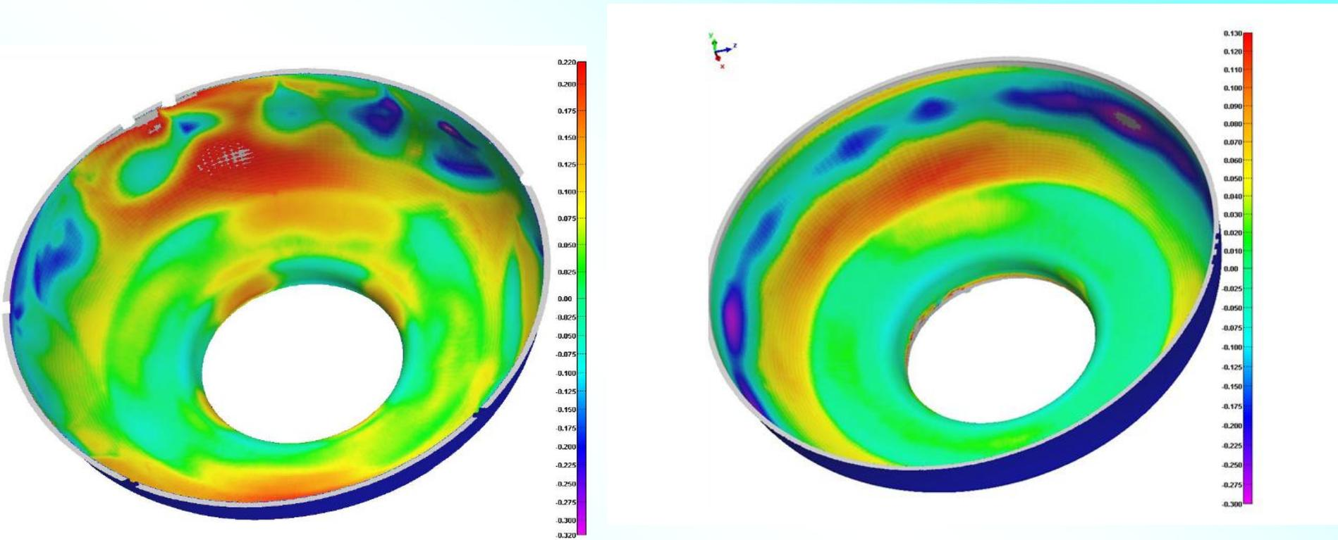
3D Image of the optical measurement of the shape on large grain half cell (left; realized accuracy  $+0,22 / -0,32$  mm) in comparison with a fine grain half cell (right; realized accuracy  $+0,13 / -0,30$  mm). The large grains are fractionally pronounced. The variation of the large grain half cell shape is somewhat larger
