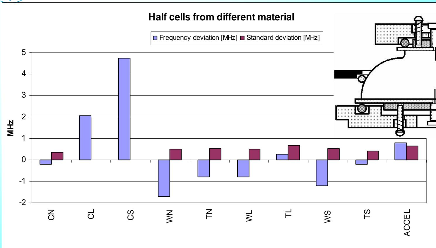
Frequency measurement of 6 end half cells (L and S) and 48 middle half cells (N) for cavities AC112-114. C - large crystal, W - Wah Chang, T - Tokyo Denkai. The shape conformity of half cells from large grain material is lower as of conventional fine grain (could be improved by correction of the tools), the uniformity of the half cells from large grain material is better.
