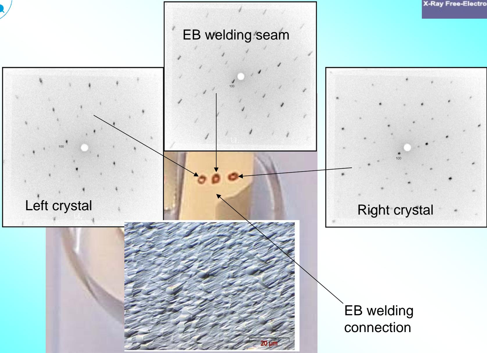
X-Ray reflexes are the same in both welded together crystals and in the welding seam
