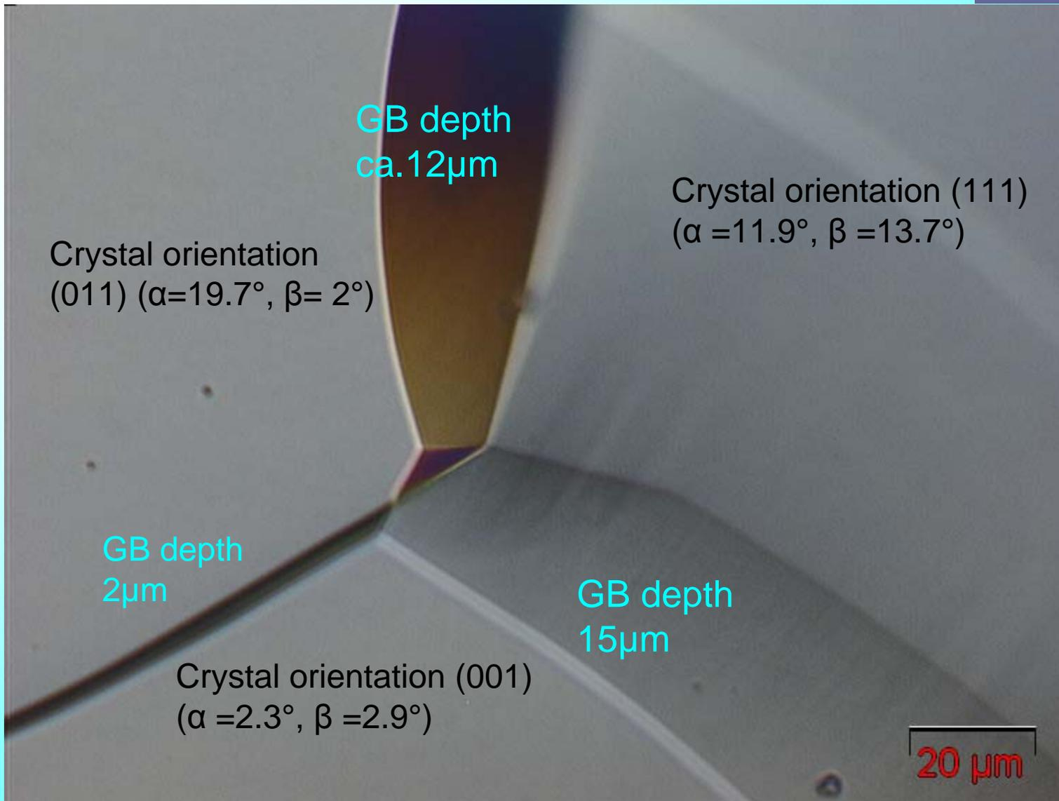
Light microscope image of LGs sample after 100 μm BCP
