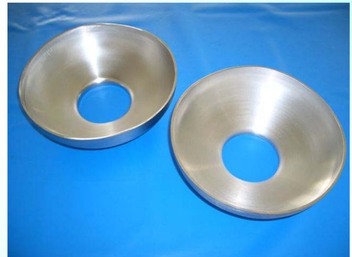
Single crystals after deep drawing at ACCEL
