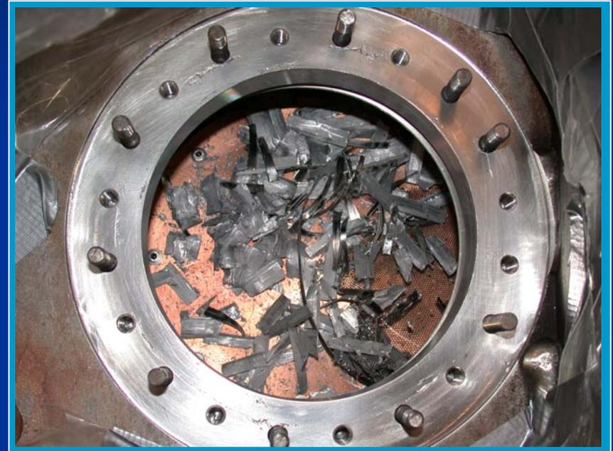
There was no time for taking the cryomodule off-line for cleaning so we removed the fragments that we could reach, vacuumed the LN2 shield, pumped down and crossed our fingers.
