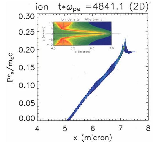
LANL simulations showing the new Break-Out Afterburner (BOA) mechanism. BOA has the potential to boost the ion energy and the acceleration efficiency by more than 2 orders of magnitude (GeV, >10%), enabling cheap, ultracompact accelerators which can be used e.g. for tumor therapy or compact plasma/field probes for large, dynamic plasma volumes.
