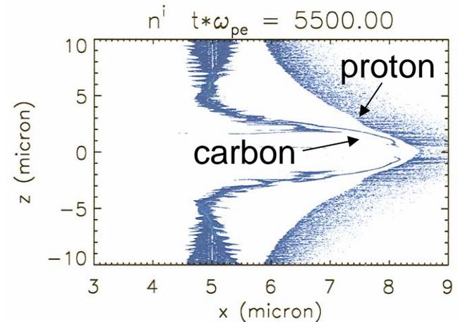
2D simulation of BOA with C target & proton layer
