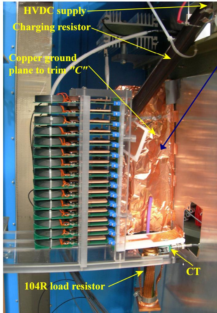
The position of the copper ground plane is changed to minimize post-pulse noise.
