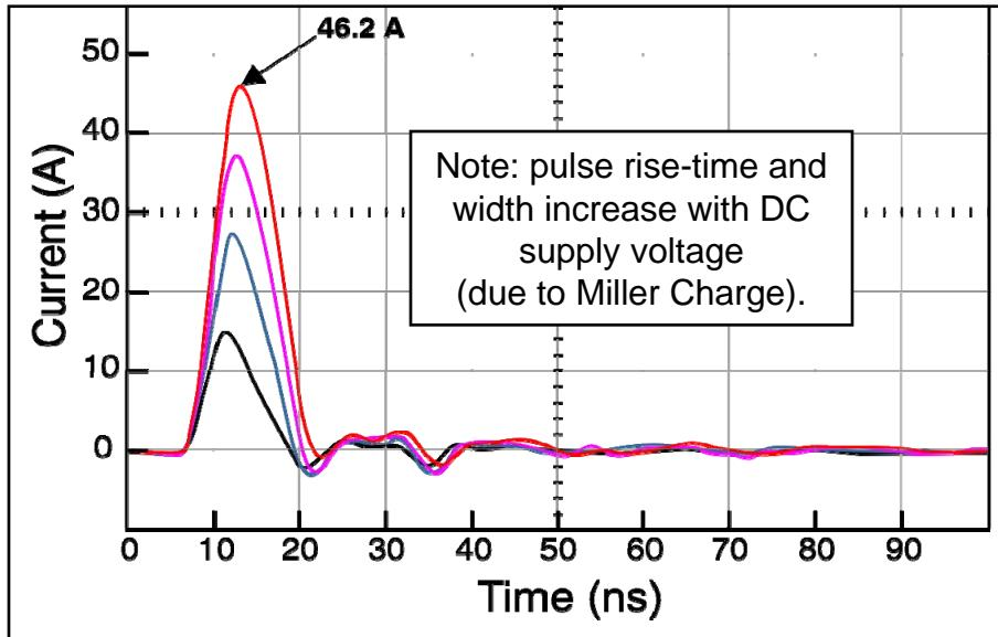
Measured pulses for 3kV, 6kV, 9kV & 12.5kV DC supply ( $C=3.3\text{pF}$ ).
