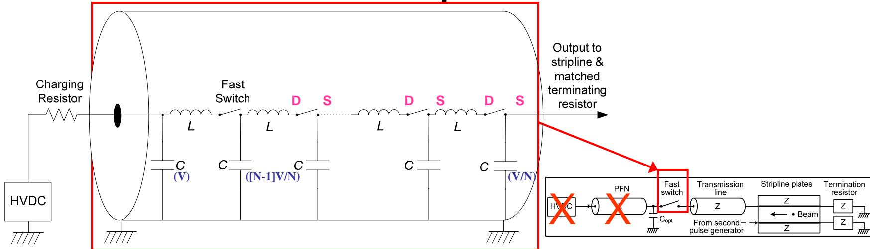
Stacked MOSFET switch is a delay line.
