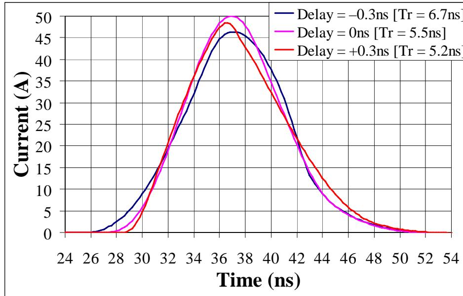
Predicted load current with -0.3ns, 0ns & +0.3ns delay between adjacent FETs (12.5kV DC).
