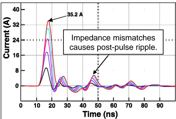
Measured pulses for 2.5kV, 5kV, 7.5kV, 10kV & 12.5kV DC supply;  $C=1.75\text{pF}$ .
