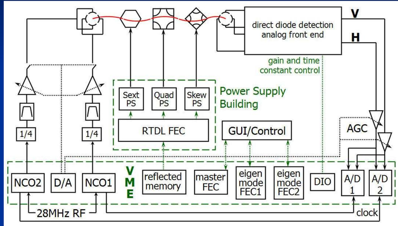
Tracking the vertical mode in the horizontal plane & vice-versa allows the coupling parameters to be calculated
