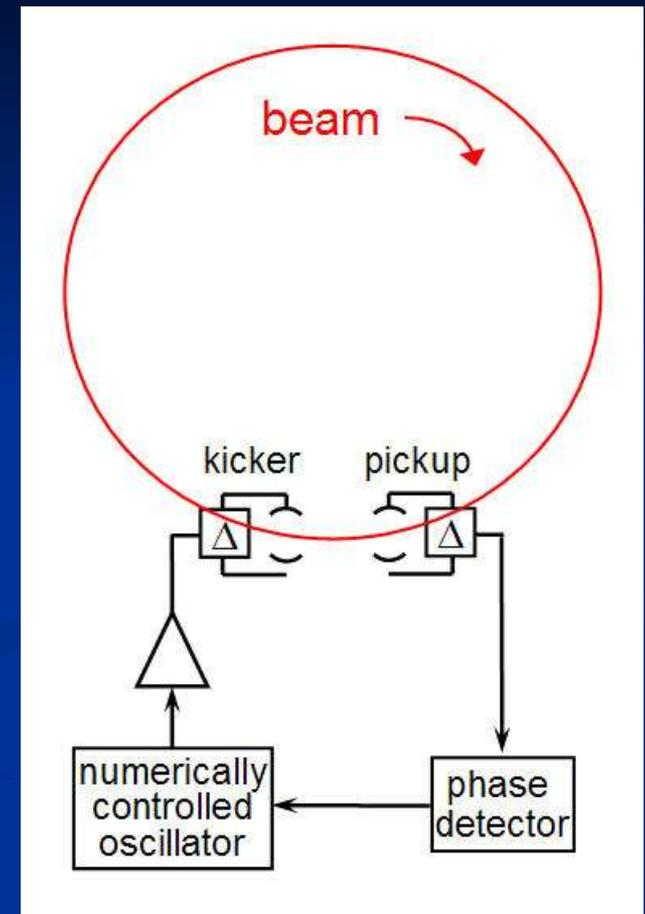
A phase-locked tune tracker comprises a continuous beam transfer function measurement at a single frequency
