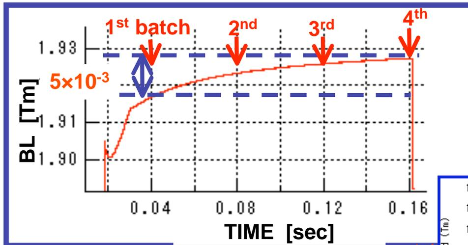
Field pattern is deteriorated due to eddy current on the magnet end. **FLATNESS** ( $\pm 5 \times 10^{-5}$ )
