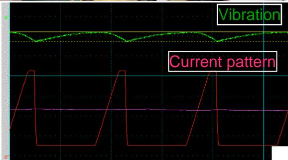
Vibration of beam duct
