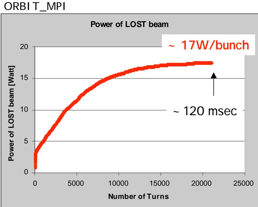
Particle losses during the acceleration for the RF pattern (40kV -> 280kV).
