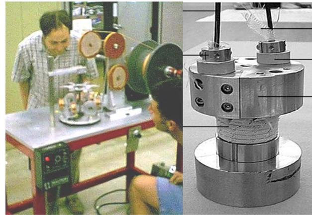
Figure 4. Fabrication and testing of structured cable: a) 6-on-1 cabling of strands onto spring tube; b) test fixture with 2.5 cm diameter winding of structured cable.
