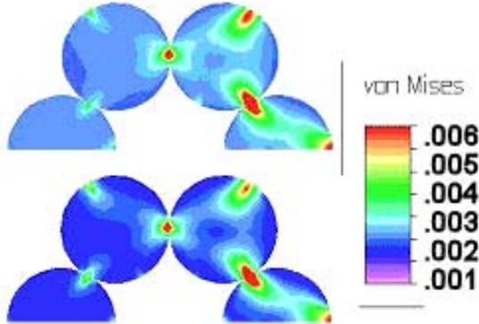
Figure 6. von Mises strain distribution in inner shell at full field: a) innermost turn; b) outermost turn.
