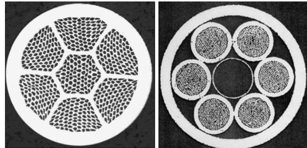
Figure 1. Bi-2212 strand and cable: a) Current high-performance Bi-2212 strand from OST; b) structured cable made using earlier strand.
