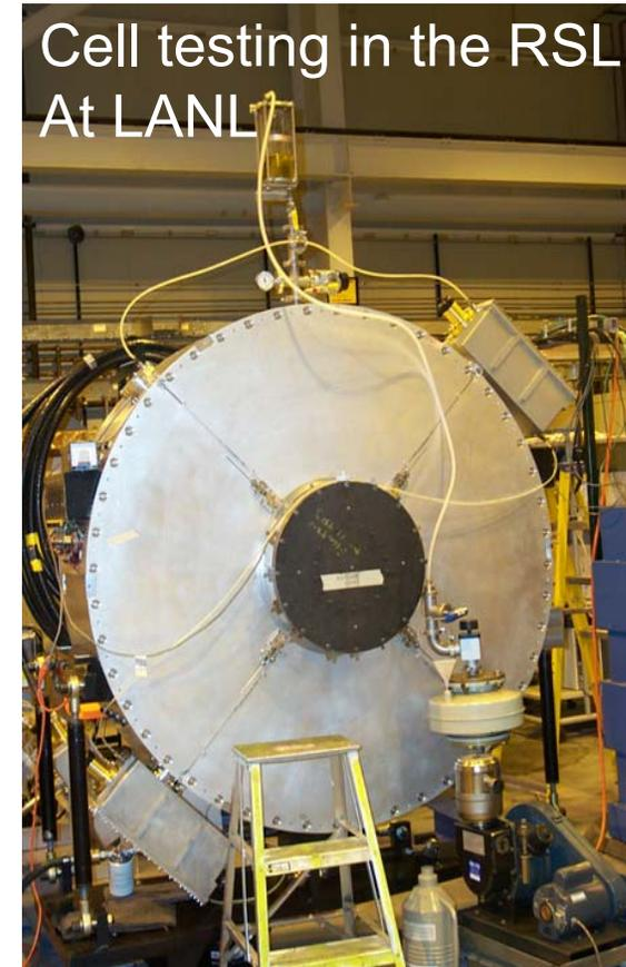
*No voltage breakdowns occurred during acceptance testing*
