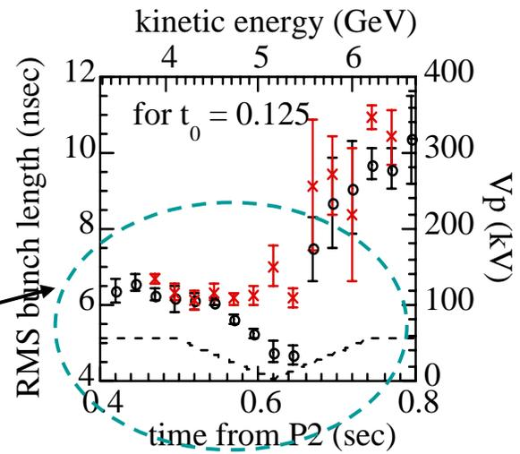
**Bunch length measured by Wall Current Monitor.**
