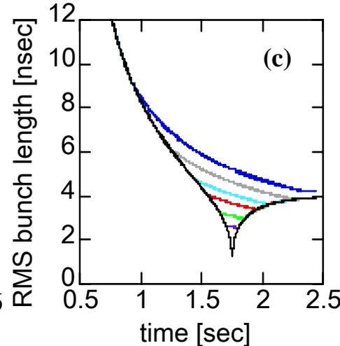
(a)  $\Delta t$  and (b)  $\Delta E$  size depend on  $n$ . (c) Bunch length control by QNTC( $n=1$ ). (sim)
