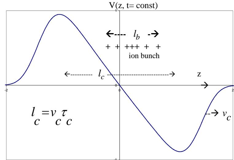
snapshot of the voltage propagating  $V(z, t=\text{constant})$
