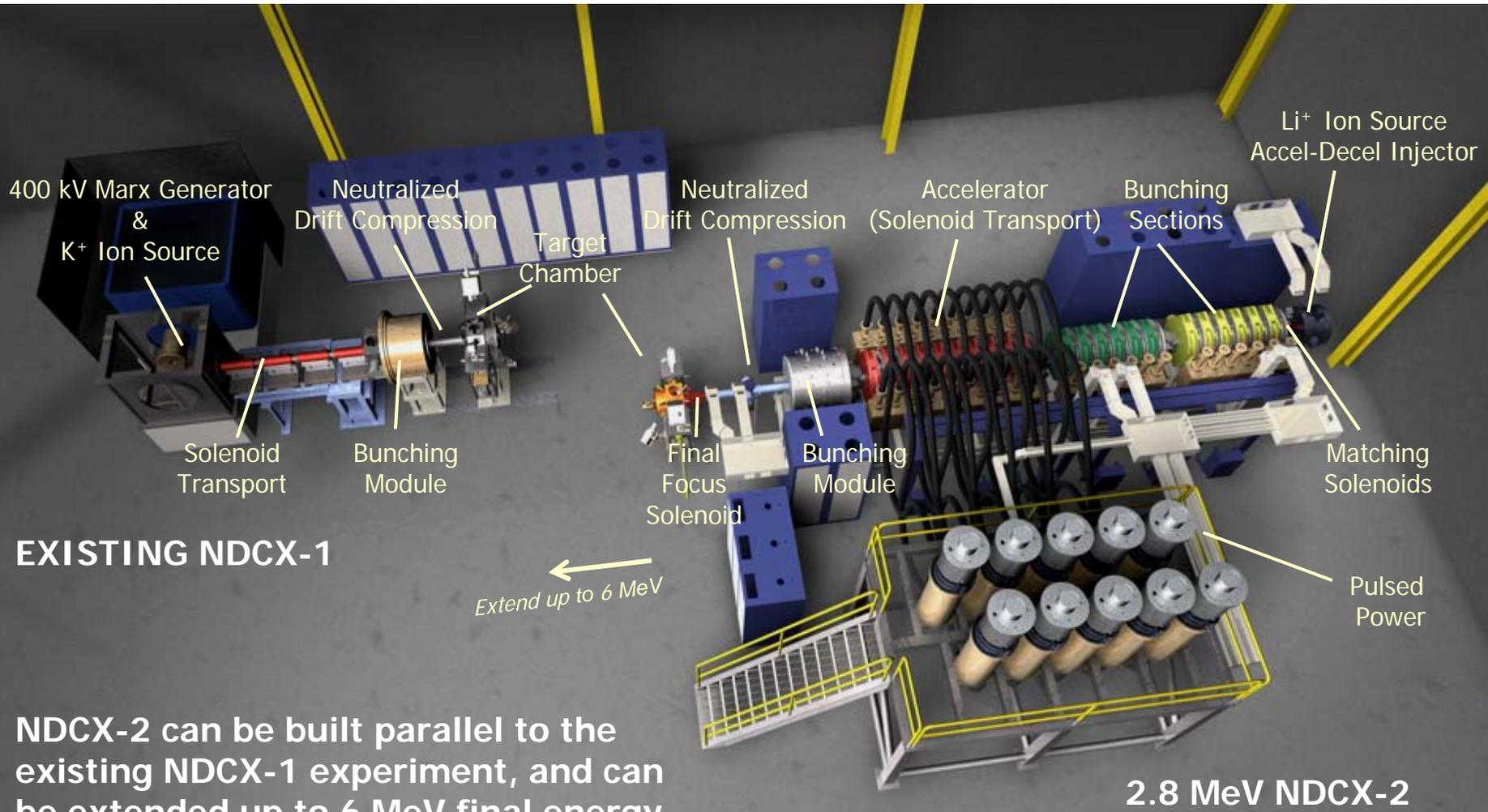
NDCX-2 can be built parallel to the existing NDCX-1 experiment, and can be extended up to 6 MeV final energy within the current building envelope.
