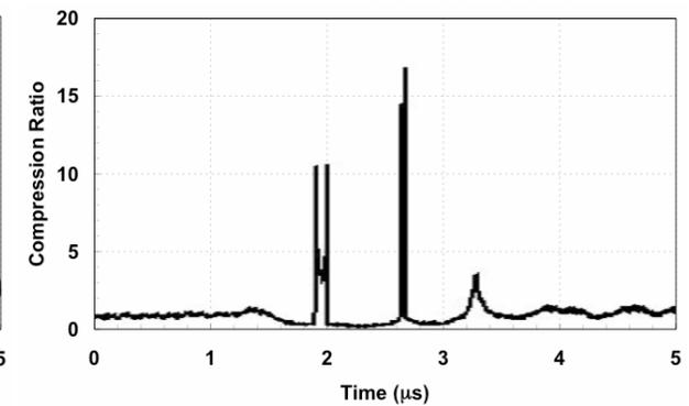
The voltage gradient was limited to  $< 2$  kV/cm by partial discharges in the vacuum. Pressure bursts and visible light were still observed during this testing, but the voltage waveform was minimally loaded and reproducible.
