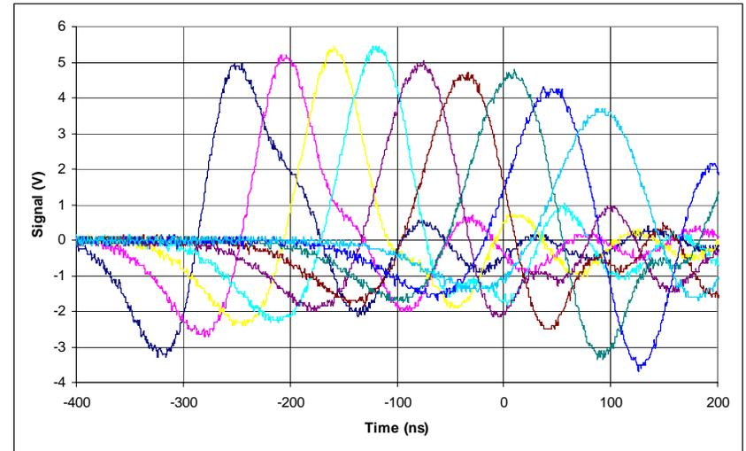
Signals from the capacitive pickups located every 10 cm along the PLIA without partial discharge (capacitive pickup signal is proportional to the time derivative of the voltage)
