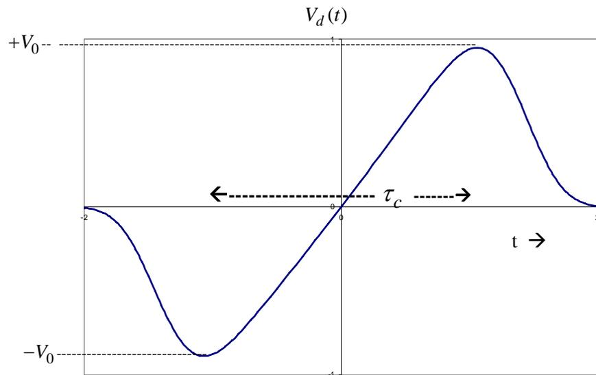
drive voltage  $V_d(t)$  applied to helix input
