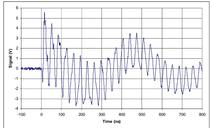
B-dot loop looking at  $B_z$  at the glass ID surface within the primary section of the helix
