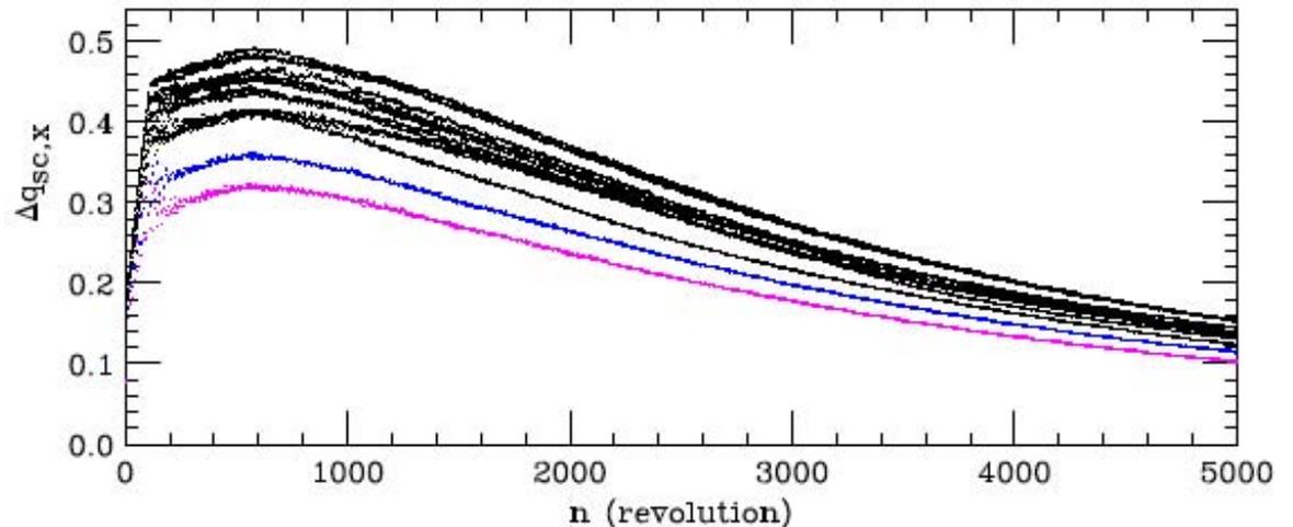
At the estimated random quadrupole error level ( $4 \times 10^{-4}$  /m), half-integer stopband causes little emittance growth.
