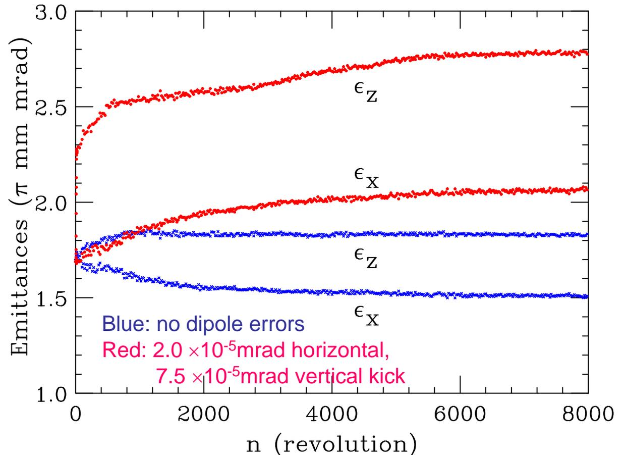
There are larger horizontal field errors (i.e. vertical kicks) than the vertical plane (horizontal kicks) because the former can easily come from dipole rolls.
