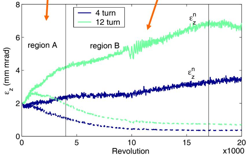
Vertical rms emittance and normalized rms emittance.
