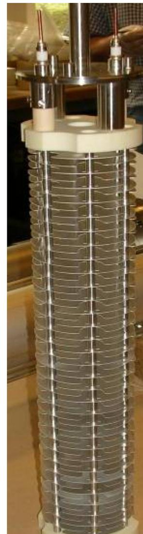
FRPMN071/72 LHC Beam Loss Measurement System
