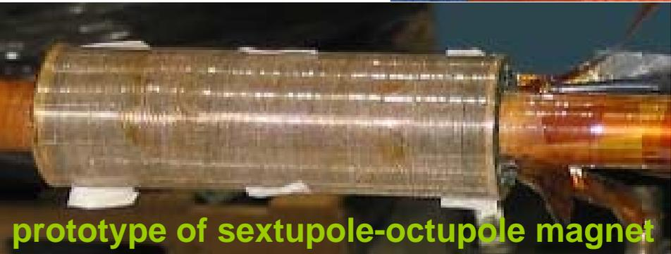
prototype of sextupole-octupole magnet
