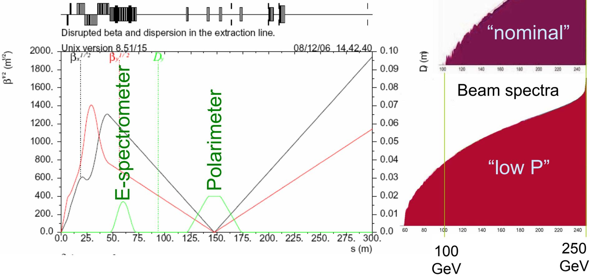
Extraction optics can handle the beam with ~60% energy spread, and provides energy and polarization diagnostics
