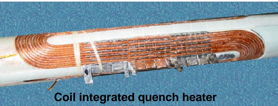
Coil integrated quench heater
