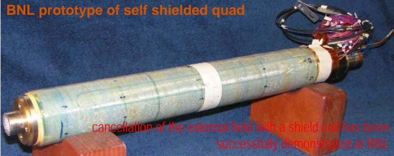
cancellation of the external field with a shield coil has been successfully demonstrated at BNL
