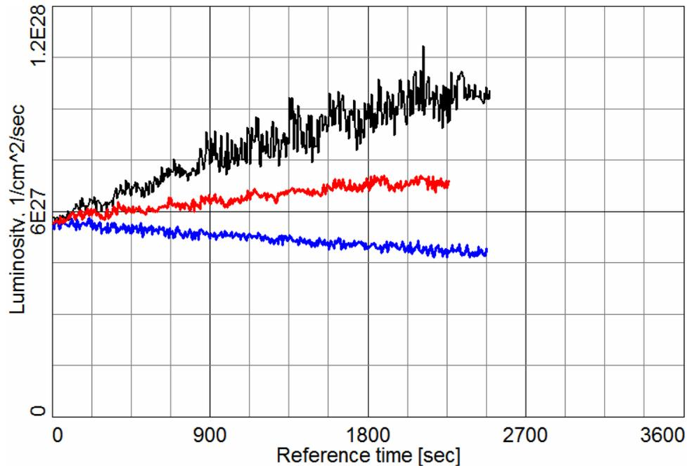
Electron cooling with realistic 6-D electron distributions. Black – using electron distribution at the start of the cooling section. Red (based on the local model) and blue (based on global parameters) using distribution at the end of the cooling section. A. Fedotov et al, High-Energy Electron Cooling Based on Realistic Six-Dimensional Distribution of Electrons. THPAS093
