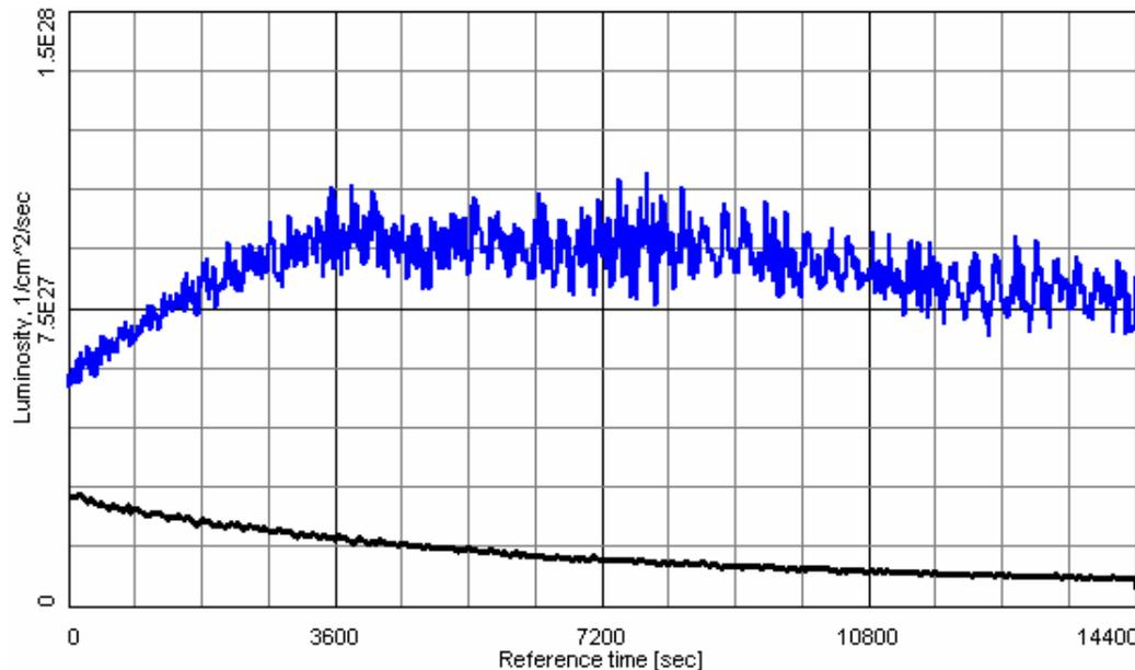
The luminosity evolution following electron cooling of 100 GeV/A gold beams at RHIC
