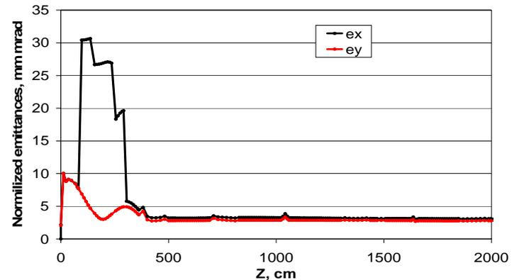
Evolution of the projected normalized transverse emittances rms in the test-bed system for beer-can distribution 5nC per bunch (final horizontal emittance black 3.1 mm mrad, vertical emittance red 2.8 mm mrad) D. Kayran et al, Optics of a Two-Pass ERL as an Electron Source for a Non-Magnetized RHIC-II Electron Cooler, THPAS096
