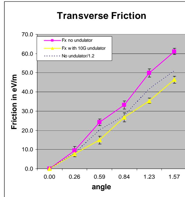
The effect of undulators on the friction force, VORPAL simulation, Red – without undulator. Yellow – with a 10 Gauss undulator. G.I. Bell et al, Numerical Algorithms for Modeling Electron Cooling in the Presence of Ext. Fields THPAS017
