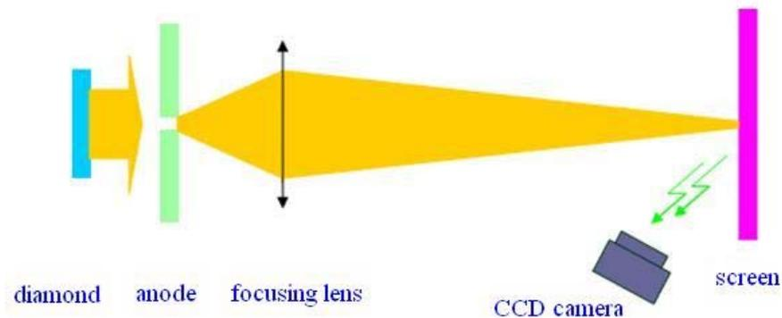
Q. Wu et al, Thermal Emittance Measurement Design for Diamond Secondary Emission
