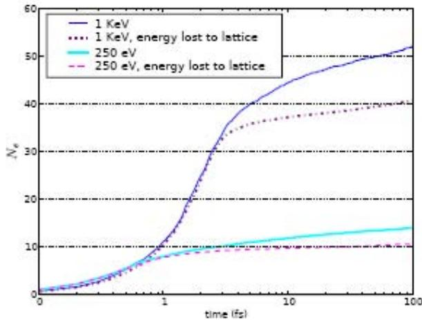
VORPAL simulation of the number of secondary electrons as a function of time following a primary impact. D. Dimitrov et al, 3D Simulations of Secondary Electron Generation & Transport in a Diamond. THPAS020
