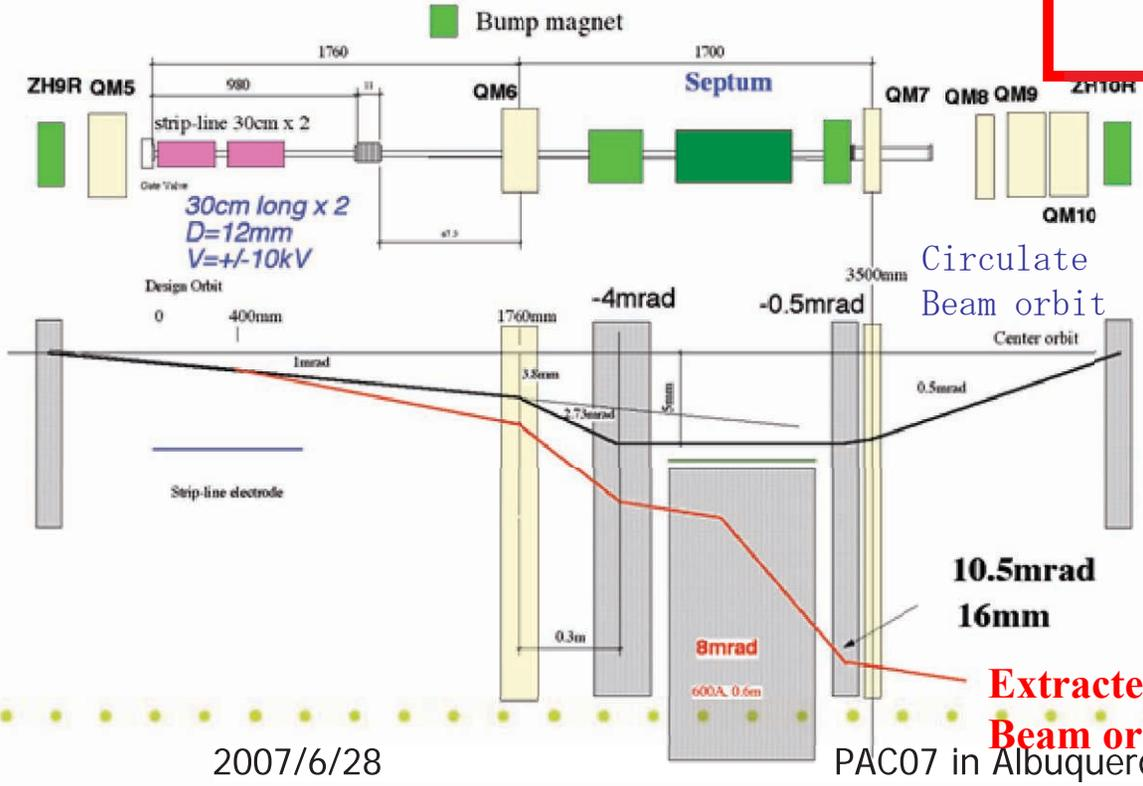
A new design uses pulse bump magnets and a thin septum magnet to help making the extraction orbit. This design makes a bump orbit after beam damping, then each beam is extracted bunch-by-bunch by the strip-line kicker.
