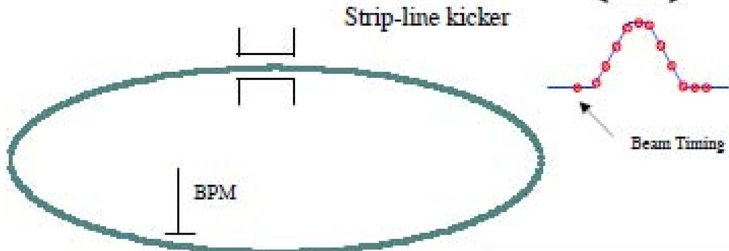
The kicker pulse is applied to the strip-line electrode at just the time of the beam goes through the electrode.
