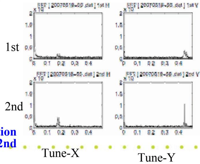
The preliminary results shows the different oscillation amplitude of the tune-X and the tune-Y for the 1st and 2nd bunches at just after injection.
