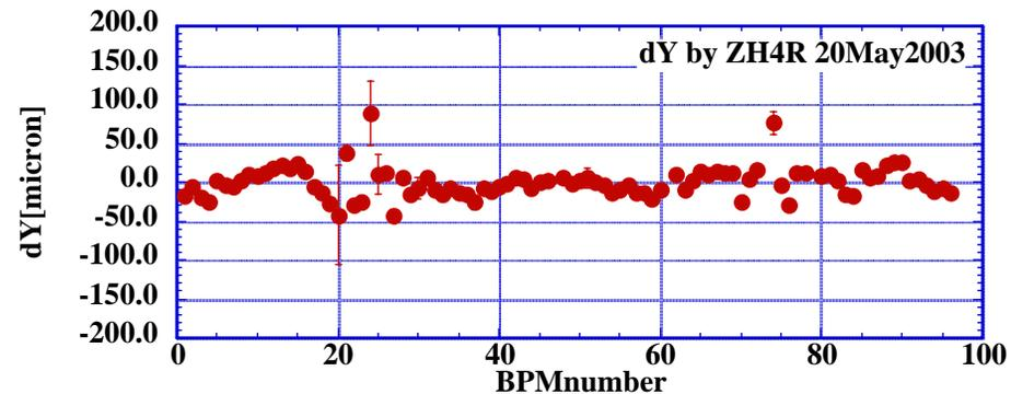
**Upgrade of BPM Resolution ( $\sim 0.1\mu\text{m}$ ) with new circuit by SLAC and FNAL. Surely, we will achieve 2pm-rad. Possibly 1pm.**
