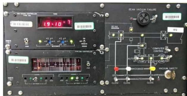
Figure 1: Hardware-based vacuum Control Chassis with adjustable vacuum set point switches.
