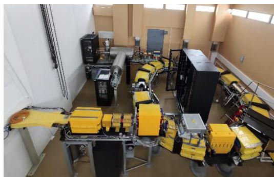
Figure 1: Protom Synchrotron-based Accelerator Complex “Prometheus” in MRRC, Obninsk, Russia.
