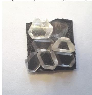
Figure 1: Synthetic crystal diamond plates.
