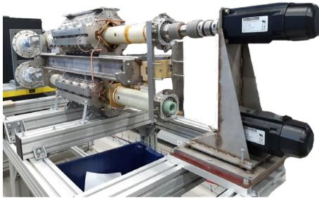
Figure 3: Warm magnetic measurement stand.
