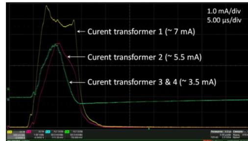
Figure 4: Current transformer signals of He<sup>+</sup> beam, 7 mA-RFQ output, 5.5 mA-IH2 output, 3.5 mA –behind QT4 triplet.
