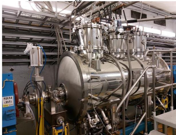
Figure 1: New 3 Tesla wiggler on Siberia-2 (SCW3).
