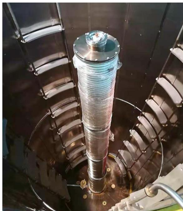
Figure 2: The ELV-15 accelerating tube.
