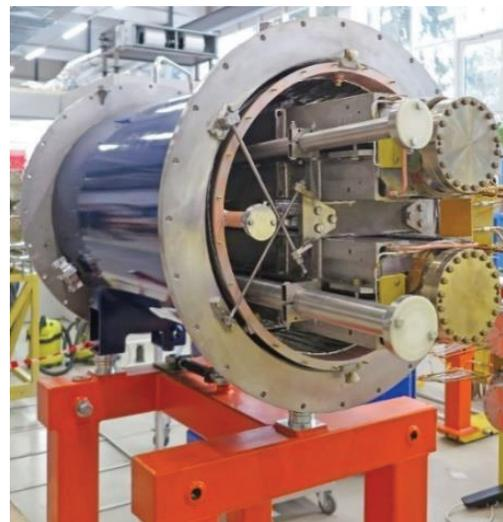
Figure 4: Collider dipole magnet.
