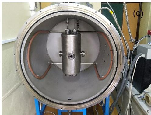
Figure 2: Niobium cavity inside of testing cryostat.
