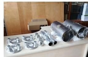
Figure 10: Nb parts for two Nuclotron-NICA cavities.
