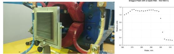
Figure 8: Aluminium ripple filter 16 mm on the left and Bragg's Peak on the right.
