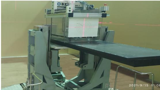
Figure 4: The 6-axis table in the medical module.
