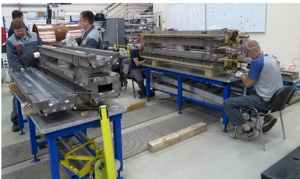
Figure 5: Preparation the magnet to cryogenic test.
