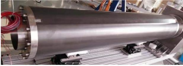
Figure 13: a prototype of CCT coil.
