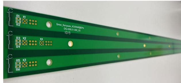
Figure 2: Block of the PCB harmonic coils.
