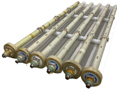
Figure 2: Serial magnetometers for collider dipole magnets.
