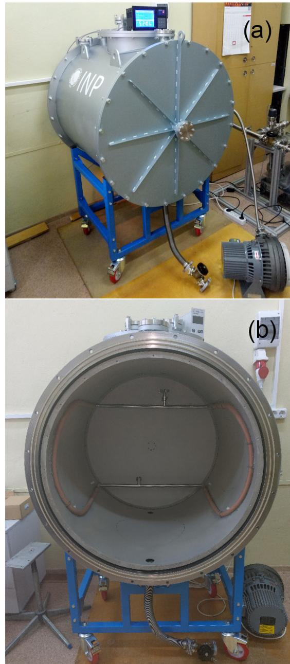
Figure 2: (a) Fabricated test cryostat, (b) the liquid nitrogen shield.
