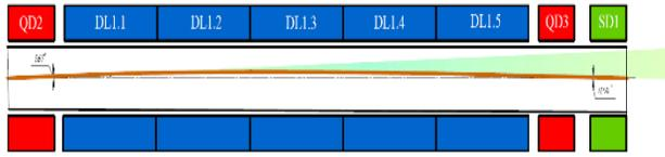
Figure 5: Synchrotron radiation of a bending magnet DL1.
