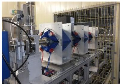
Figure 3: The beginning section of the HILAC-Booster beam transport channel.
