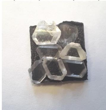
Figure 1: Synthetic crystal diamond plates.
