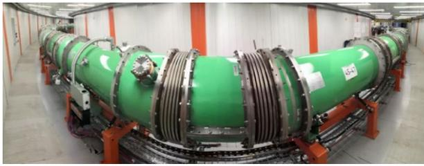
Figure 7: Booster ring inside Synchrohasatron yoke.
