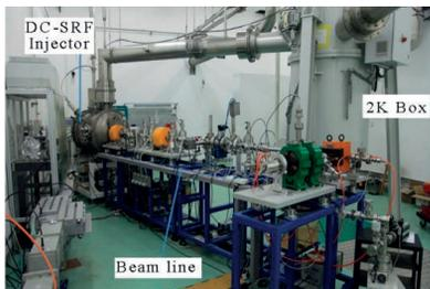
Figure 2: Beam line of the 3.5-cell DC-SRF injector.
