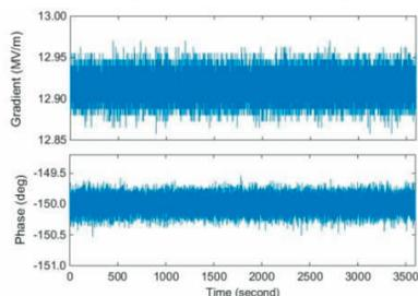
Figure 3: Long-term running of LLRF control system.
