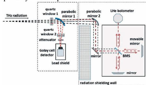
Figure 7: Schematic of the THz measurement system.
