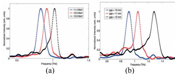
Figure 14: Measured THz spectra with different electron beam energies (a) and undulator gaps (b).
