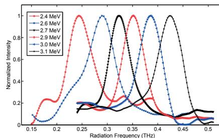
Figure 8: Measured THz spectra with different electron beam energies.
