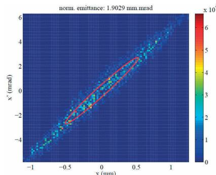
Figure 4: measured emittance of electron beam.
