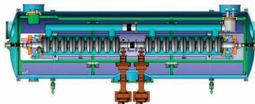
Figure 12: The sectional view of 2×9-cell SRF linac.
