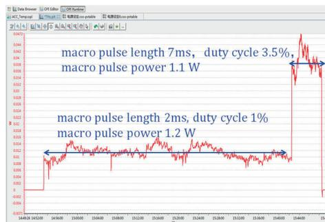
Figure 15: Measured THz power at different macro pulse.
