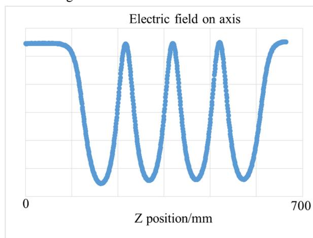
Figure 3: The electric field distribution of the fundamental mode in the 4-cell cavity.
