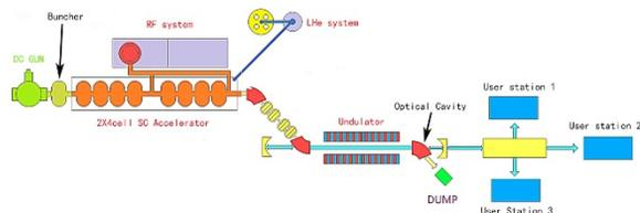
Figure 1: Layout of the CAEP THz-FEL facility.
