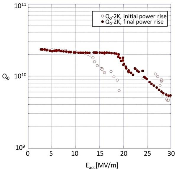
Figure 5:  $Q_0$  versus  $E_{acc}$  for a 4-cell cavity at 2 K temperature.
