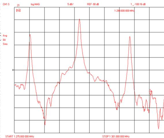
Figure 4: The  $S_{21}$  parameter of the HOM coupler.
