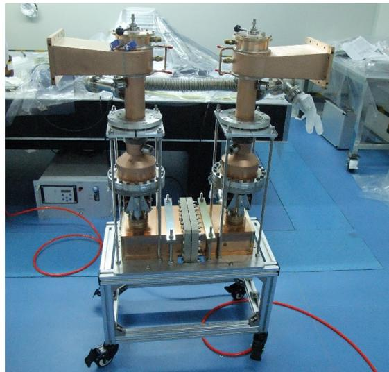
Figure 6: The conditioning structure equipped with couplers.
