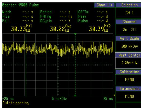
Figure 7: The max power reaches 30 kW in CW mode.
