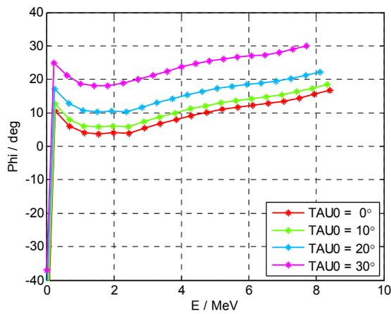
Figure 2: Phase slip of particles in central region.
