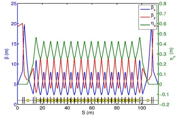
Figure 1: Optical functions and lattice structure of quarter.
