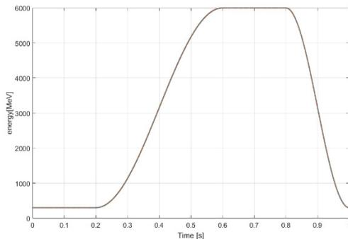
Figure 4: An energy ramp cycle in the booster.
