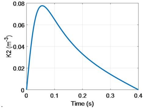
Figure 5: The sextupole strength induced by eddy current in ramping up process.
