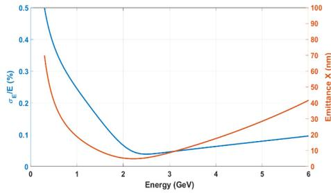
Figure 7: Emittance and energy spread evolution in ramping.
