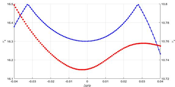
Figure 3: The chromaticity curves of HEPS booster lattice.
