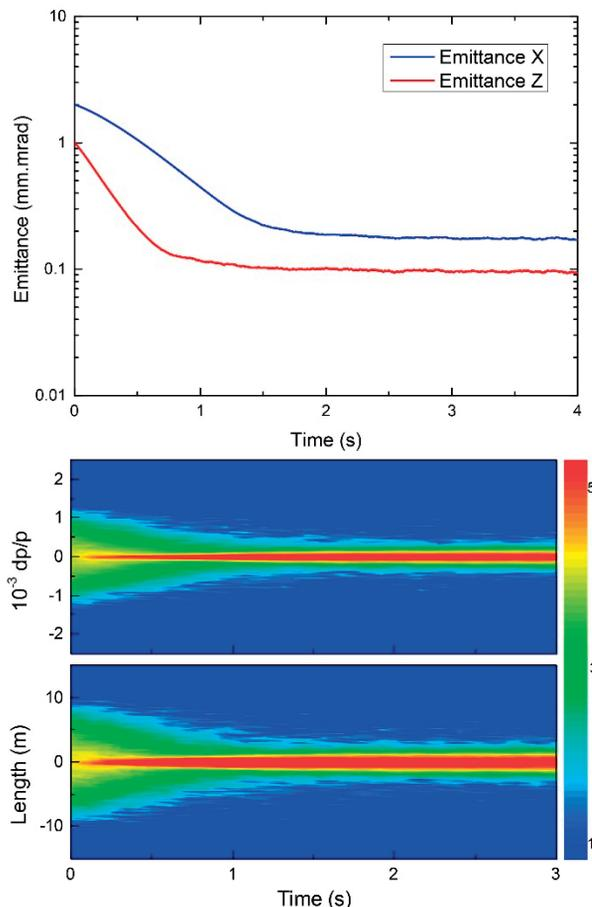
Figure 1: Evolution of beam emittance (RMS), distribution of momentum spread and bunch length in the procedure of cooling combined with RF field ( $V_{RF}=1.0$  kV for 6.9 MeV/u C beam).
