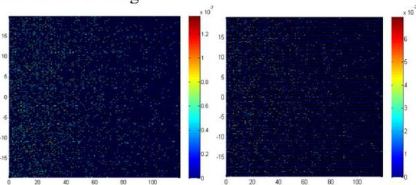
Figure 5: left: energy deposition of gamma; right: energy deposition of neutron.
