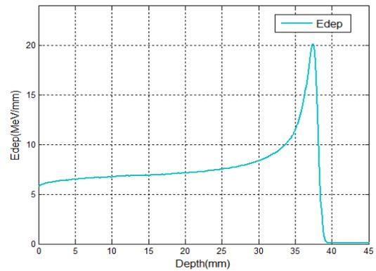
Figure 3: Energy deposition curve of  $250\text{MeV}$  proton beam in tungsten.
