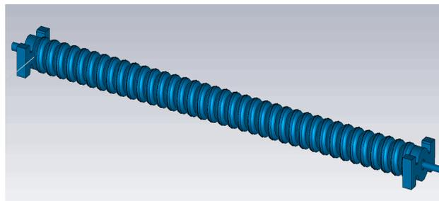
Figure 5: Completely electromagnetic model of S-band TW tube.
