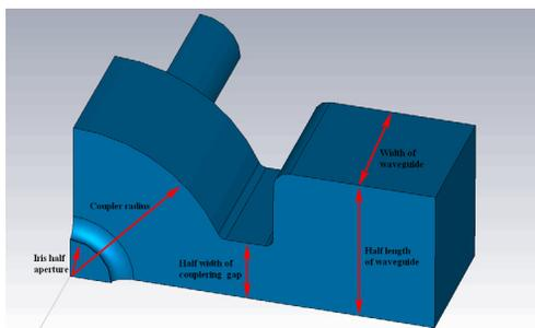
Figure 3: Symmetric split of coupler model in simulation.
