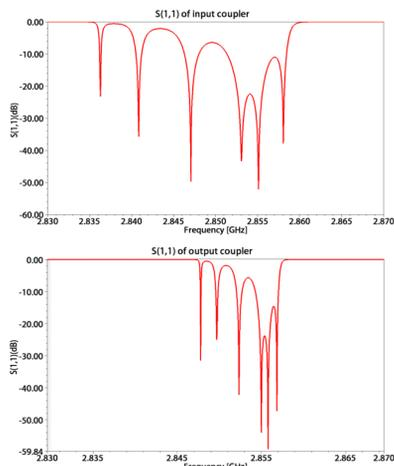
Figure 4: S (1, 1) parameter of input/output coupler.
