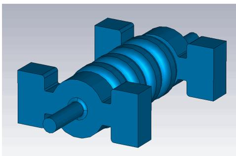
Figure 2: Model of coupler with four cells.
