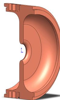
Figure 6: Mechanical model of individual cavity design.
