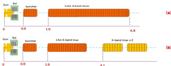
Figure 1: Present linac layout and upgrade proposal.
