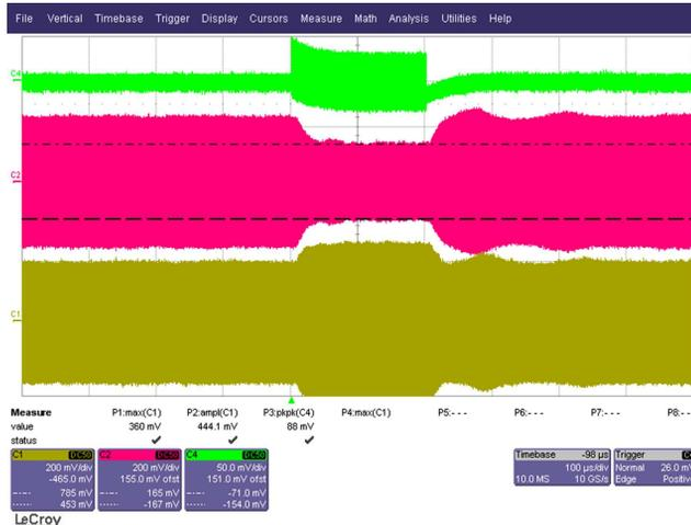
Figure 5: Beam current signal (green), reflected signal (red) and forward signal (yellow) in pulse mode.
