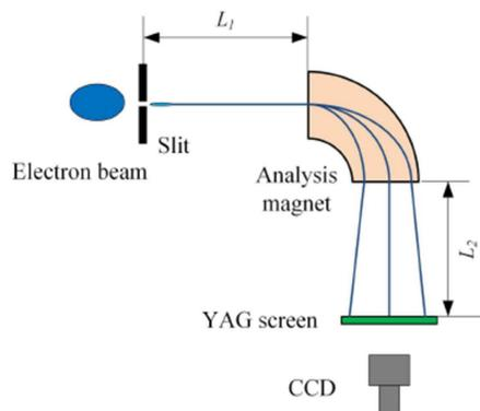
Figure 6: The energy and energy spread measuring principle.
