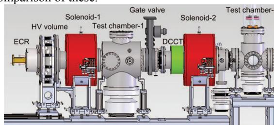
Figure 2: The layout of the LEBT of C-ADS.
