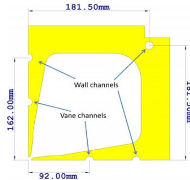
Figure 9: The water cooling channels.
