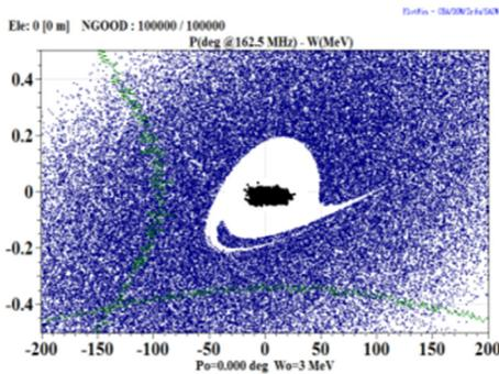
Figure 4: The 99.9% longitudinal emittance and longitudinal acceptance of super conducting section.
