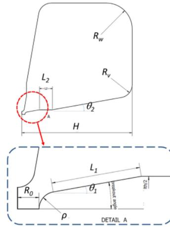
Figure 5: The cross section of CMIF RFQ.
