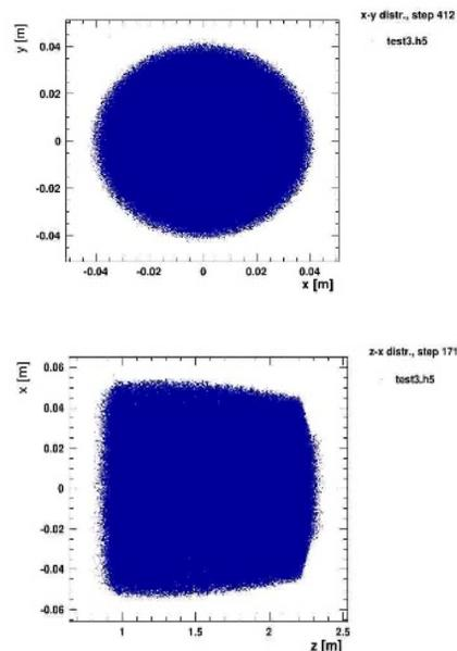
Figure 7: Initial particles space at injector exit for a 2.6 MeV, 2 kA and 1000 mm-mrad beam.
