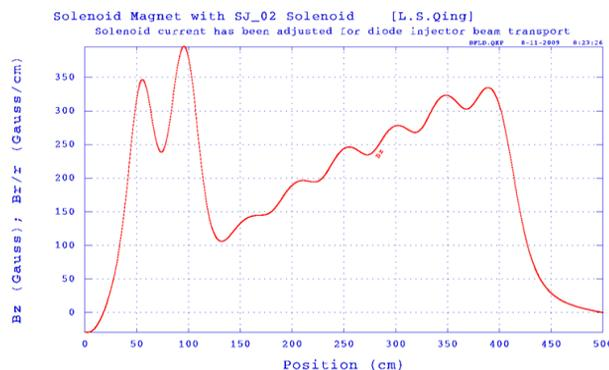
Figure 2: The axial magnetic field of the Injector.
