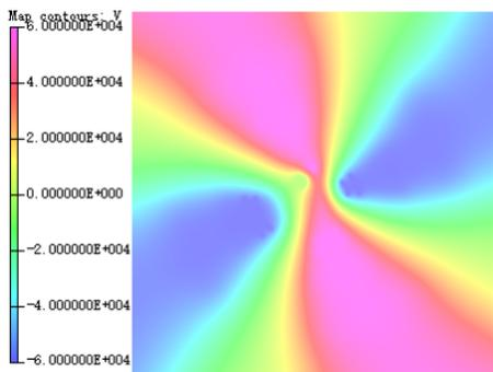
Figure 3: Potential distribution diagram calculated by TOSCA.
