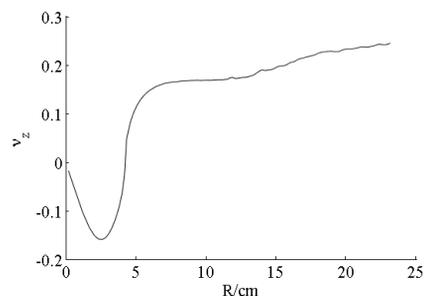
Figure 5: Radial distribution of the vertical focusing tunes.
