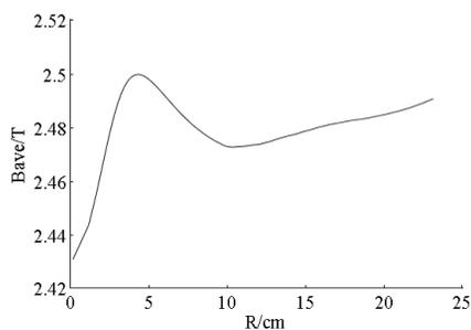
Figure 4: Radial distribution of the central region average magnetic field.
