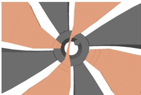
Figure 2: Structure diagram of the central region electrode.
