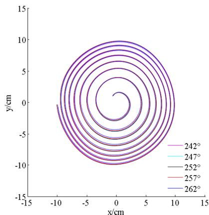
Figure 6: Particle orbit diagram for the initial phase ranging from 242° to 262°.
