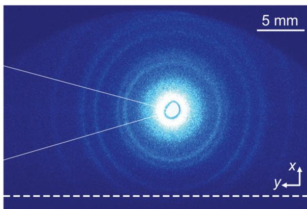
Figure 2: A single-shot MeV UED diffraction pattern.
