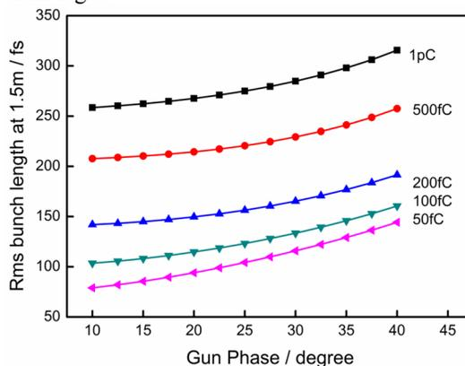
Figure 4: Bunch length vs launching phase.
