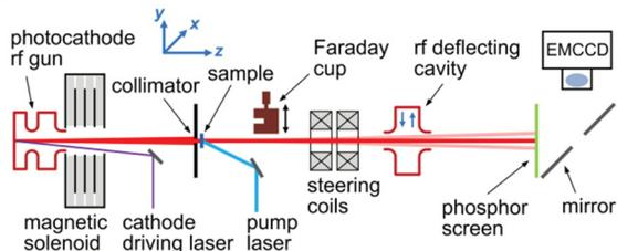
Figure 1: Schematic of the MeV UED system.
