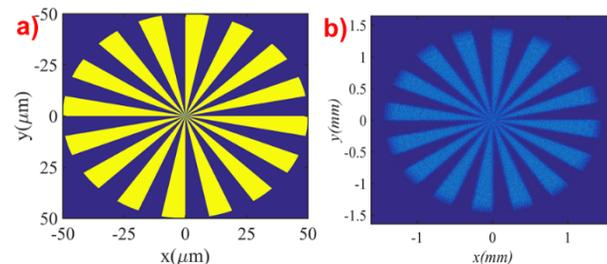
Figure 5: a) distribution of the virtual sample; b) image of a virtual sample with ~30 times magnified.
