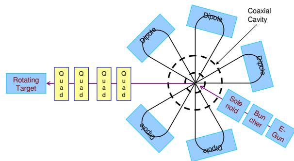
Figure 1: Layout of the proposed micro-focused X-ray source.
