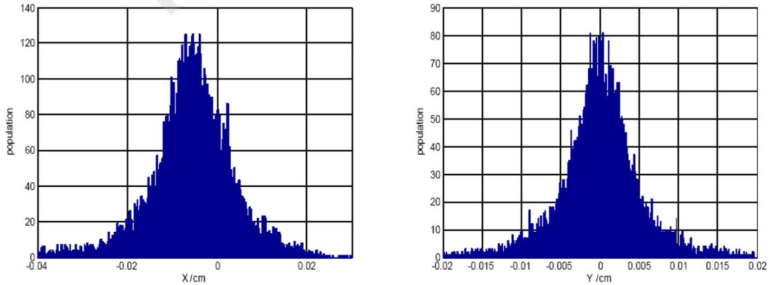
Figure 3: Distribution of the electron focus spot in x and y direction.
