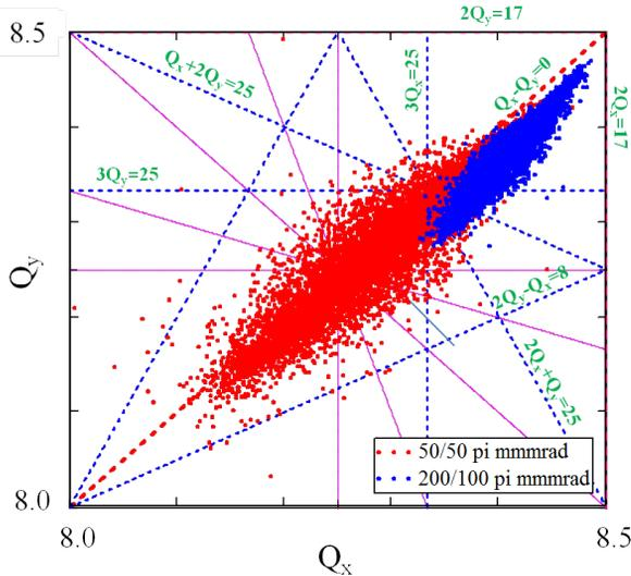
Figure 2: Resonances in tune diagram at the BRing i.e., linear difference coupling (red dotted line),  $3^{rd}$ -order betatron (blue dotted line),  $4^{th}$ -order structure (pink solid line), and two half-integer resonances; The nominal working point for  $^{238}\text{U}^{35+}$  injection is set as (8.45, 8.43).
