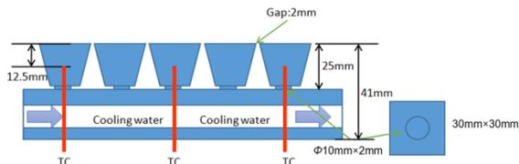
Figure 2: The design of short-pulse diagnostics calorimeter.
