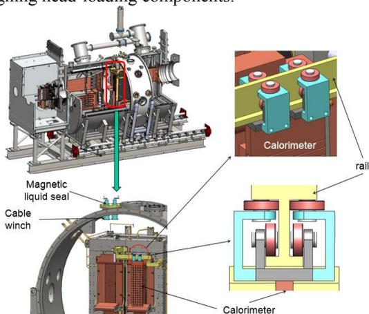
Figure 1: The layout of short-pulse diagnostics calorimeter.
