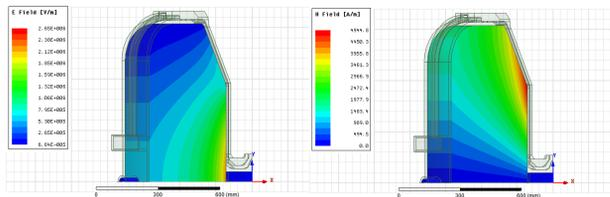
Figure 2: Electric field and magnetic field intensity. The cavity wall dressed with water cooling jacket appears as the transparent portion.
