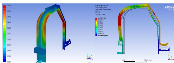
Figure 7: Updated temperature rise and induced deformation, note the frame in solid line is undeformed.
