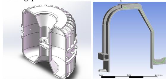
Figure 4: Left: Full cavity mechanical model; right: reduced model for coupled simulation, the water volume is coloured in green.
