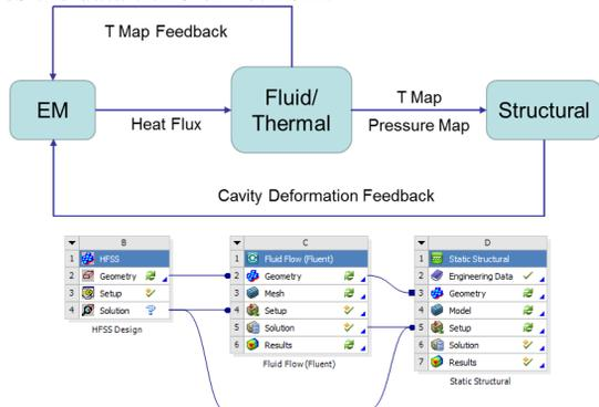
Figure 3: The work flow of the coupled analysis and a snapshot in ANSYS user interface.
