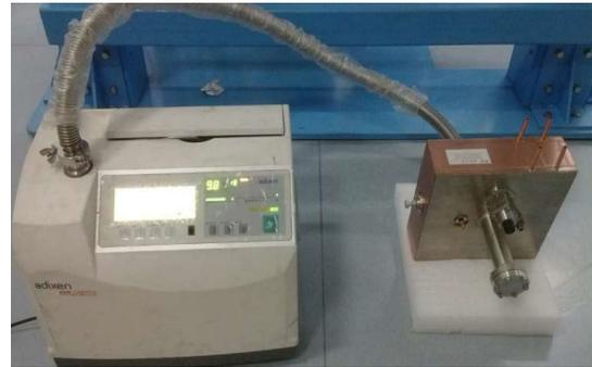
Figure 3: The vacuum leak detection of the cavity.
