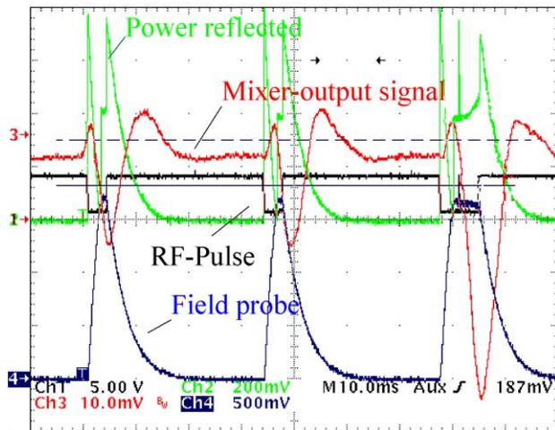
Fig. 5: Phase behaviour (mixer output signal) of the test cavity during an additional long pulse at an accelerating field of 5MV/m
