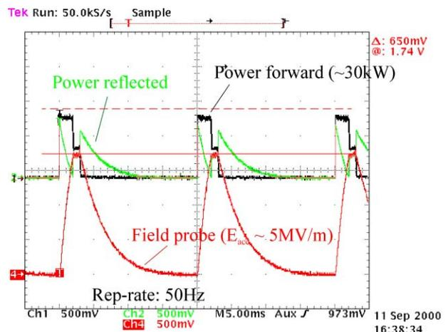
Fig.1: Pulsed operation of the ESS Test-Cavity
