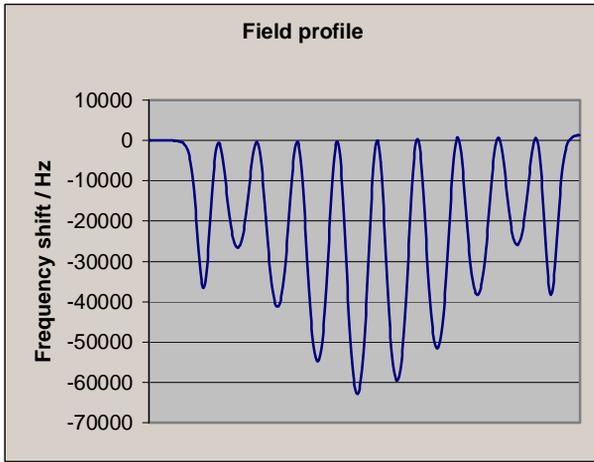
Fig. 7: Field profile of a copper 10-cell spoketype cavity
