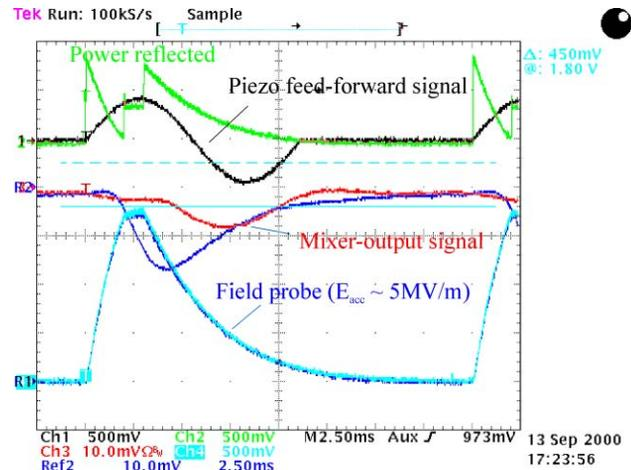
Fig. 6: Compensation of Lorentz force detuning with piezos elements. Additionally, the mixer output signal without piezos correction is drawn for comparison.
