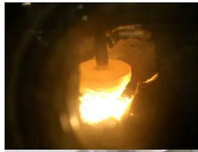
EB melting of ingot
