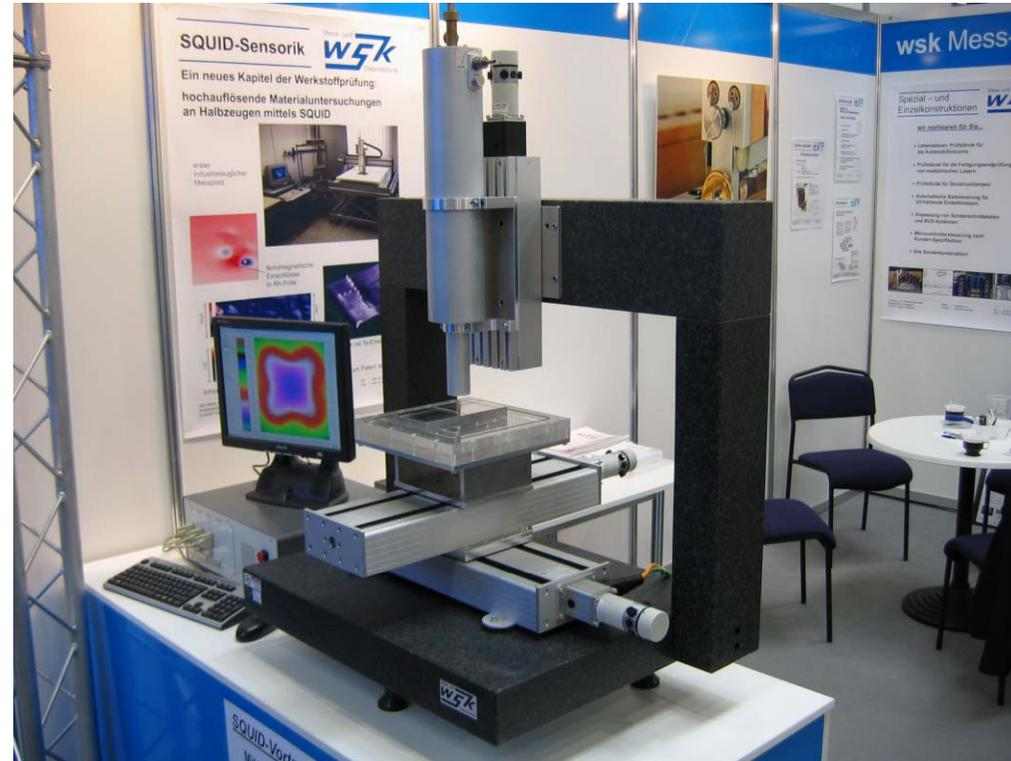
An excitation coil produces eddy currents in the sample, whose magnetic field is detected by the SQUID.
