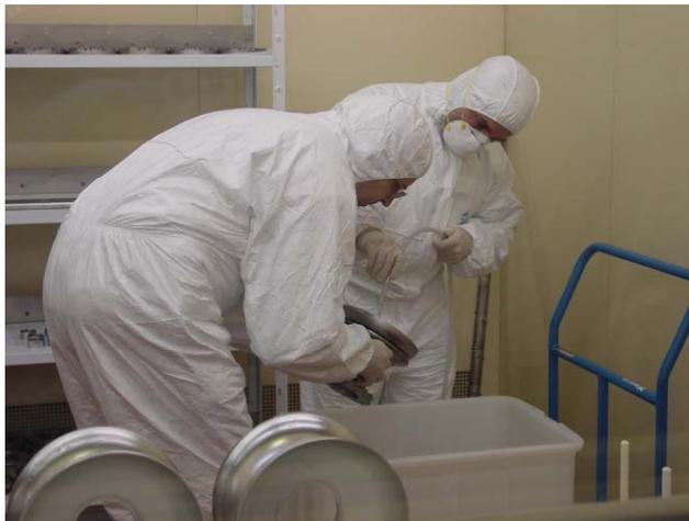
1. Degreasing and rinsing of parts
