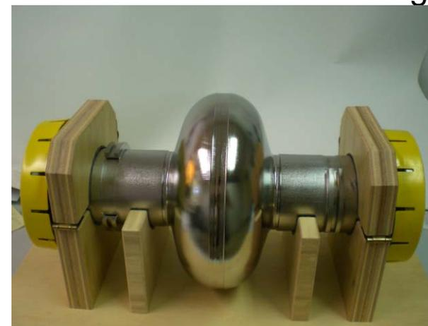
DESY SC cavity 1AC8 (TESLA shape) build from Heraeus disc by rolling at RWTH, deep drawing and EB welding at ACCEL
