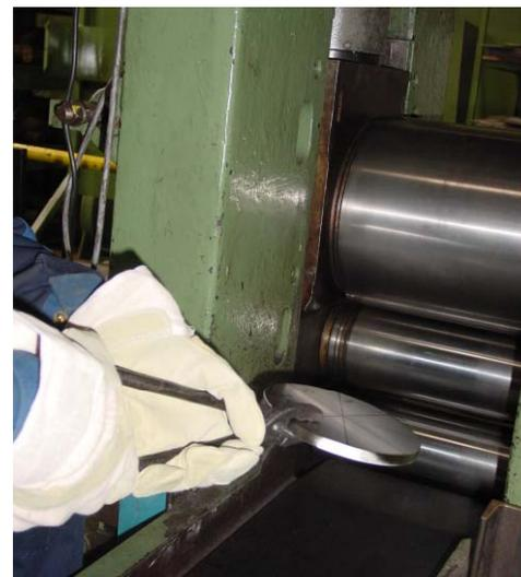
3. Increasing of diameter by special rolling with an intermediate annealing
