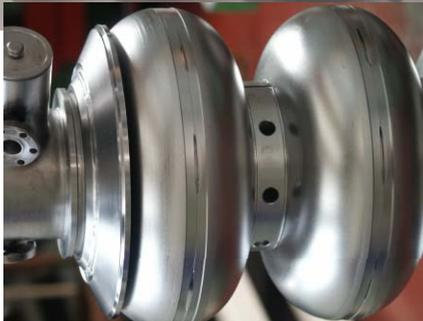
After proper cleaning eight dumb bells and two end group sections welded by electron beam together
