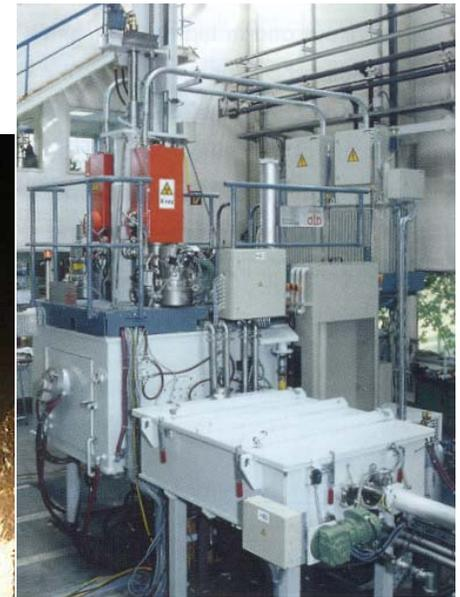
EB furnace for melting of refractory metals
