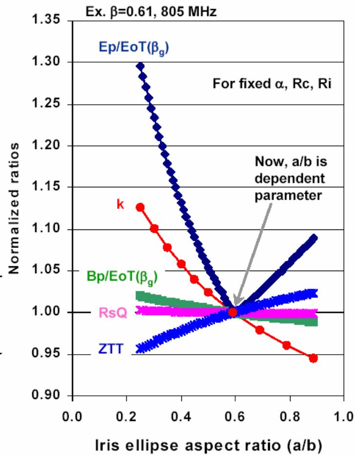
Elliptical cell geometry and dependencies of RF parameters on the ellipse aspect ratio ( $a/b$ ) at the fixed slope angle, dome radius and bore radius.
