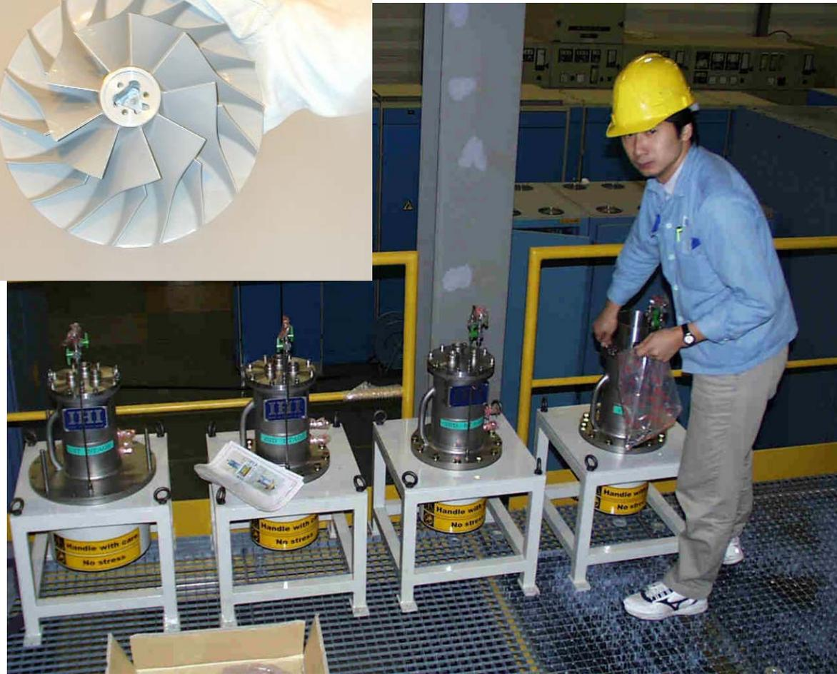
The four-stage LHC cold compressors
