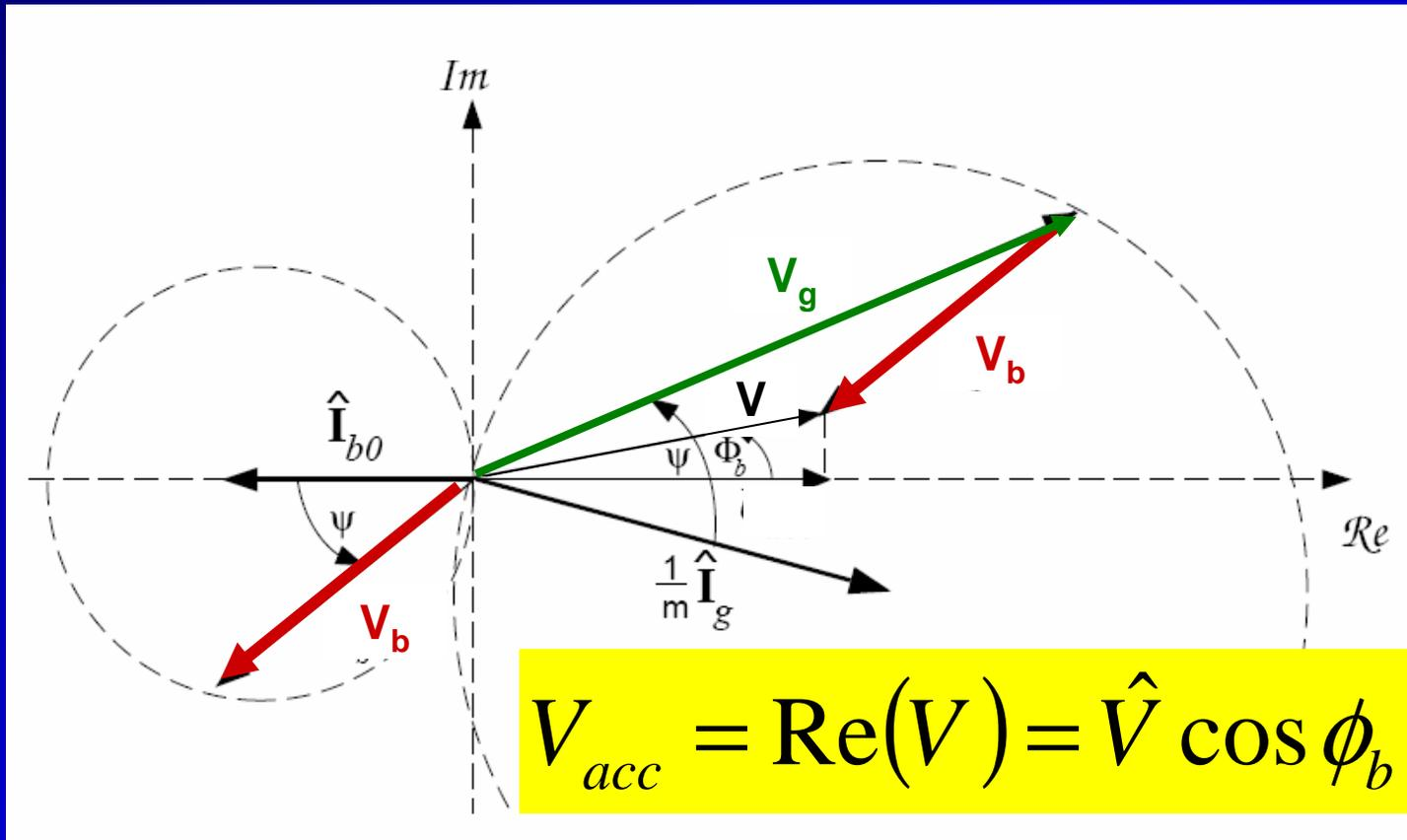
$$\Psi = \tan^{-1} \left( \frac{\Delta \omega}{\omega_{1/2}} \right) = \text{tuning angle}$$
