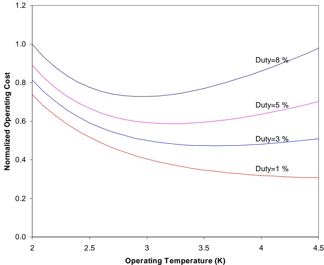
For SNS, operation at 4.2 K is overall more economical up to about  $\frac{1}{2}$  of the design beam power (if achieved by reducing repetition rate to 30 Hz)
