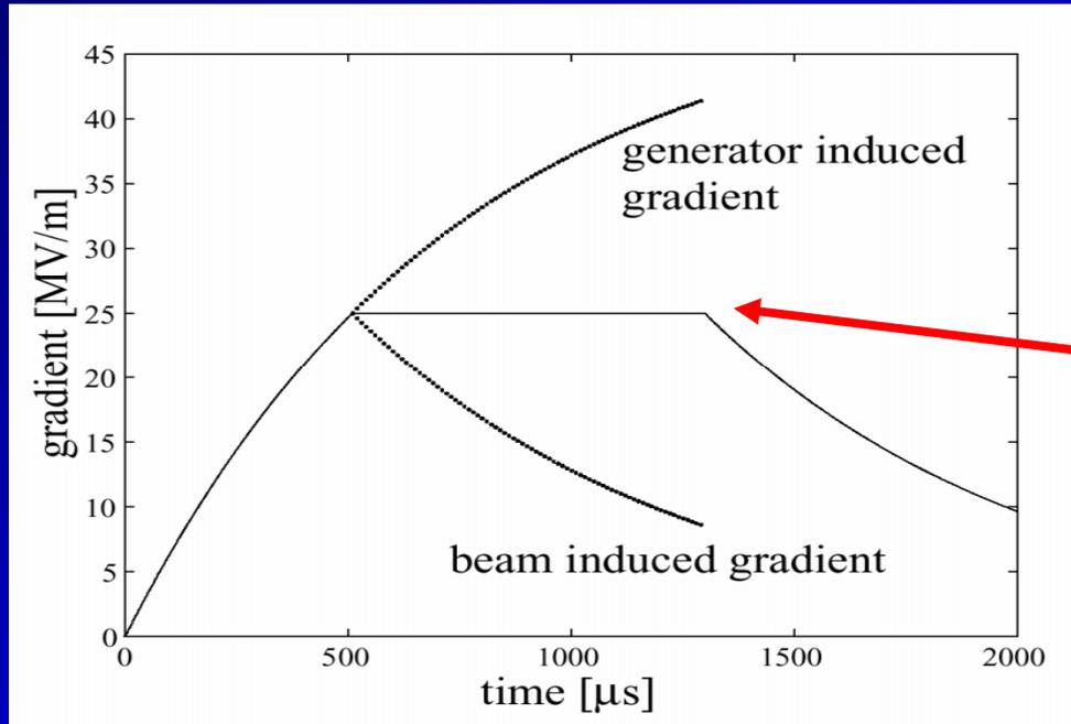
The generator and the beam induced voltage compensate each other if  $Q_L$  is properly adjusted.
