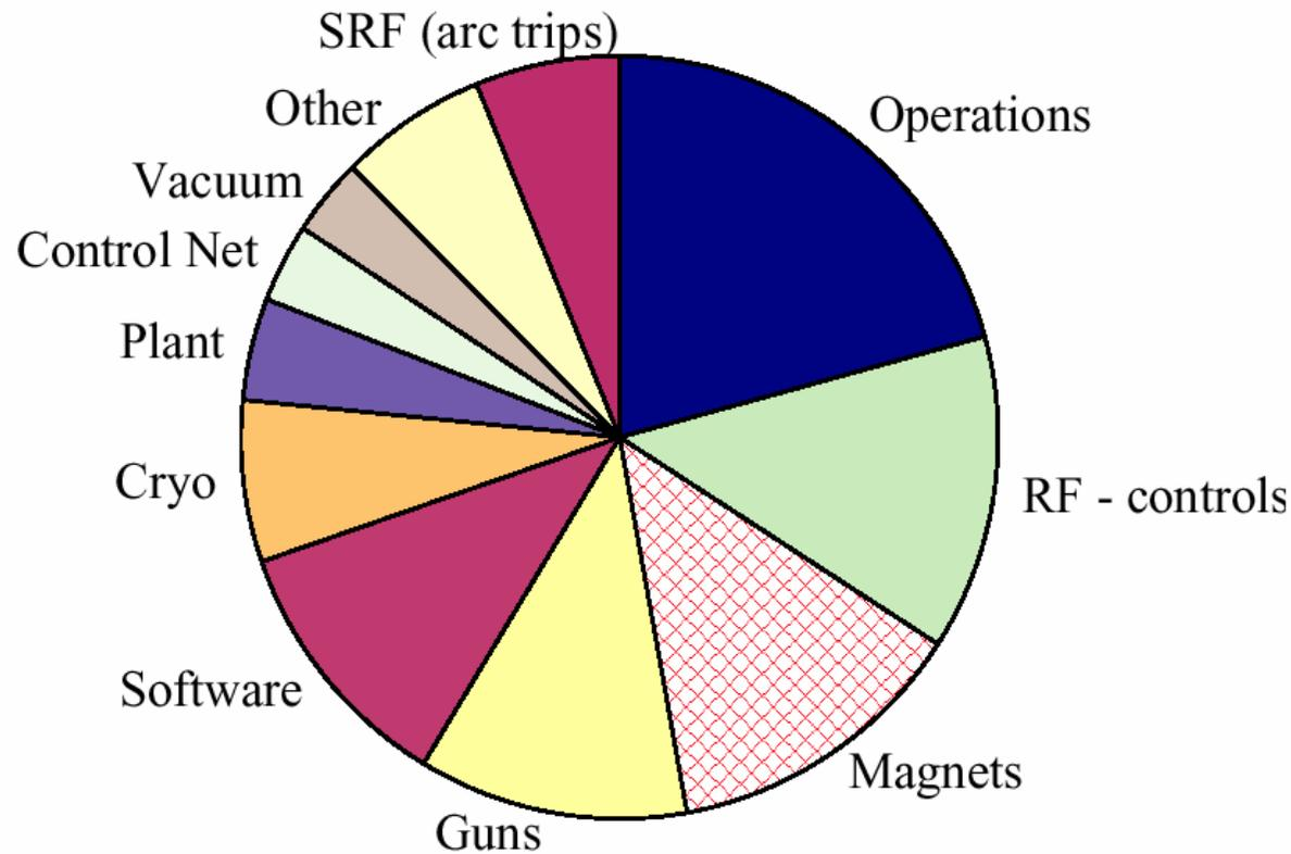
**Other than the arc trips, the SRF system directly contributed 48 minutes (less than 0.1%) of the 1620 hours of unscheduled downtime.**
