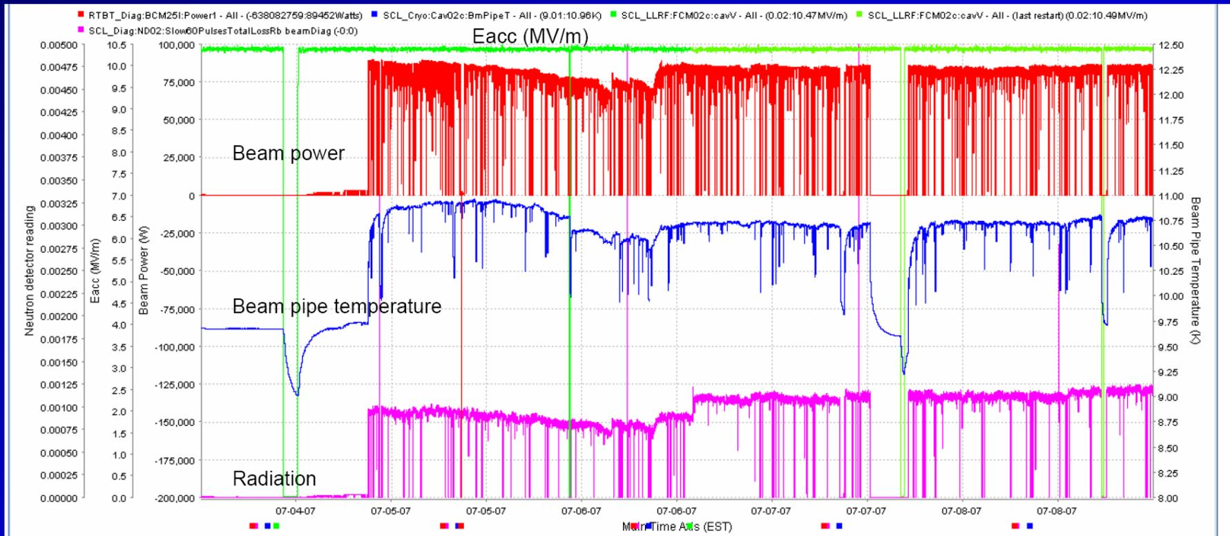
Beam pipe temperature increases by beam induced heating
