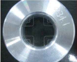
Figure 3: The grid in a mockup drift tube.
