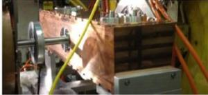
Figure 1: The new copper buncher.
